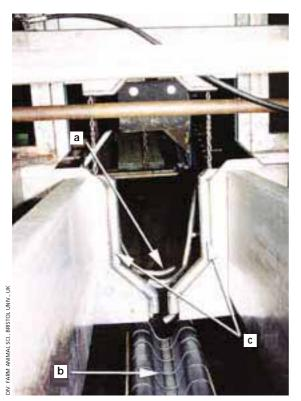
PHOTO 7.3 Upright cattle restraint with monorail (internal view) a) Chin lift, b) Monorail, c) Neck restraint welfare problems may be common, especially when handling cattle.
