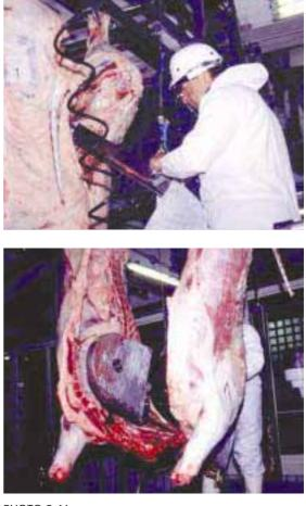
**PHOTO 8.46** Splitting the carcass in the medial plane by power saw
