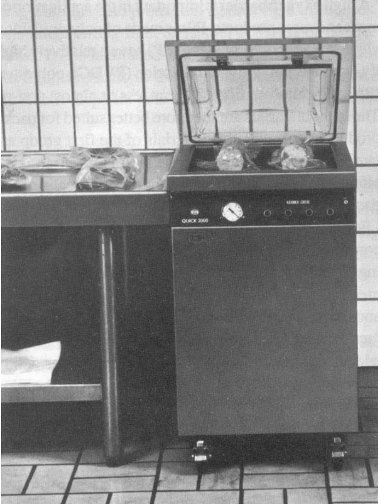
Longer storage times for traditionally preserved dried meat can be achieved with vacuum-packaging in laminated films, which protect against humidity and
