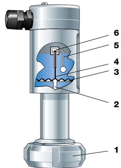
**Fig. 7.13** Pressure transmitter
