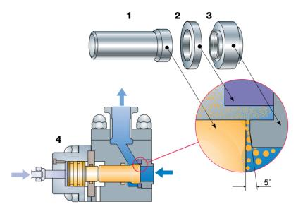
**Fig.6.3.5** The components of a single-stage homogenisation device.
