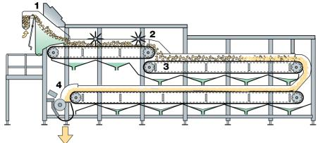
**Fig. 14.21** Continuous cheddaring machine with three conveyors, suitable for Mozzarella cheese.
