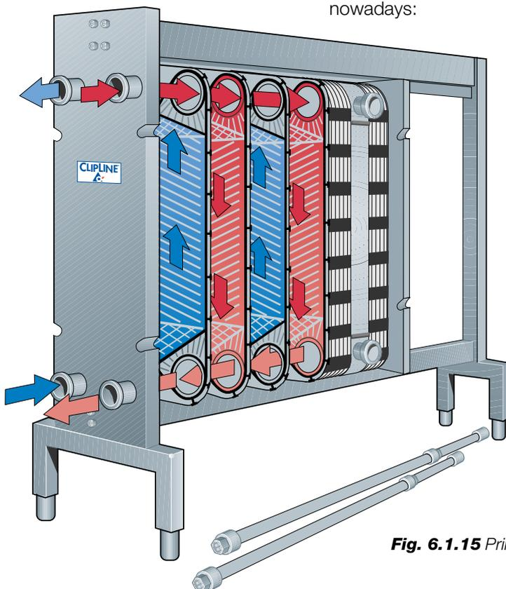
**Fig. 6.1.15** Principles of flow and heat transfer in a plate heat exchanger.
