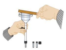
Fig 11.8 The SMR viscosimeter.
