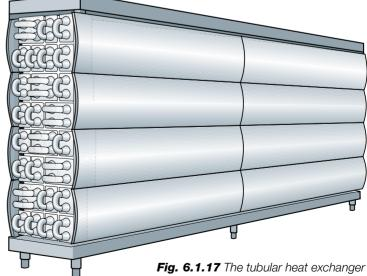
tubes are assembled in a compact unit.
