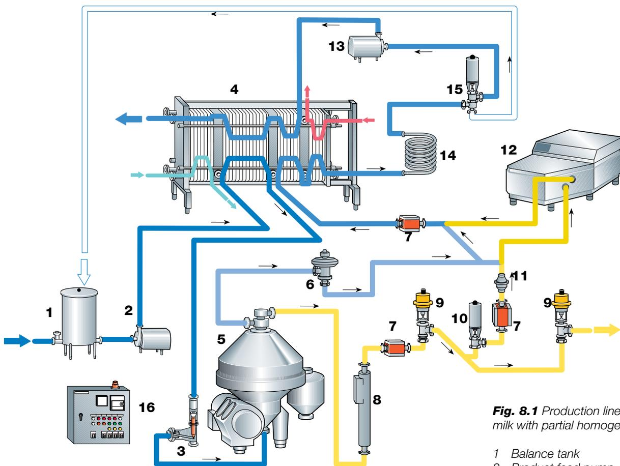
**Fig. 8.1** Production line for market milk with partial homogenisation.
