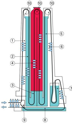
**Fig. 9.10** Hydrostatic vertical continuous bottle steriliser
