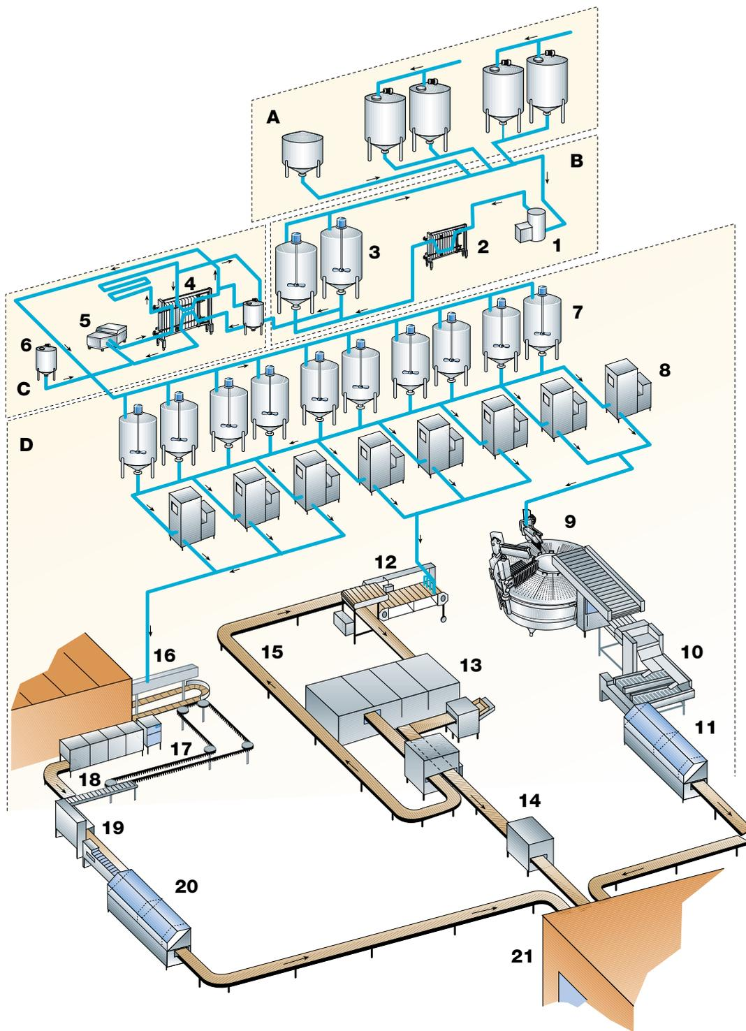
**Fig. 19.10** Large ice cream plant for production of 5 000–10 000 l/h of various types of ice cream.
