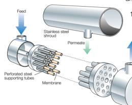
**Fig. 6.4.5** Example of a tubular module to be integrated into a UF (or RO) system (PCI).
