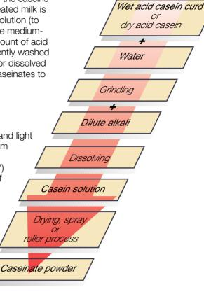
Fig. 20.5 Basic steps involved in the manufacture of spray or roller dried caseinates from acid casein curd or dry acid casein. Alkali may be sodium hydroxide, potassium hydroxide, calcium hydroxide, or ammonia.
