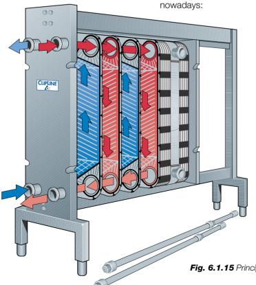
Fig. 6.1.15 Principles of flow and heat transfer in a plate heat exchanger.
