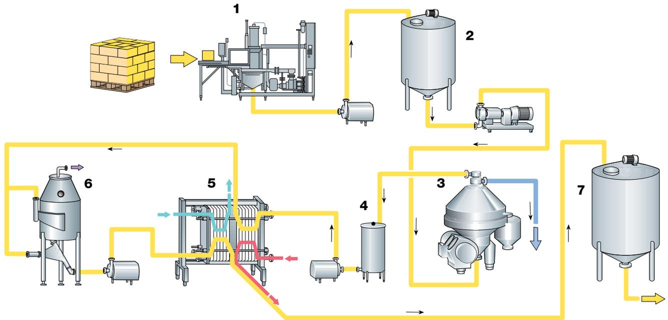
**Fig. 13.4** Production line for AMF from butter.
