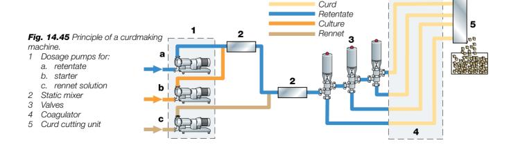
filled. The proper coagulation time in the pipes is controlled by the speed of the dosing pump.
