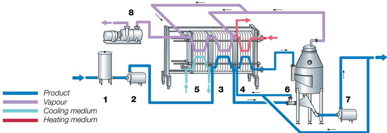
**Fig. 6.5.2** Process line for a circulation evaporator.
