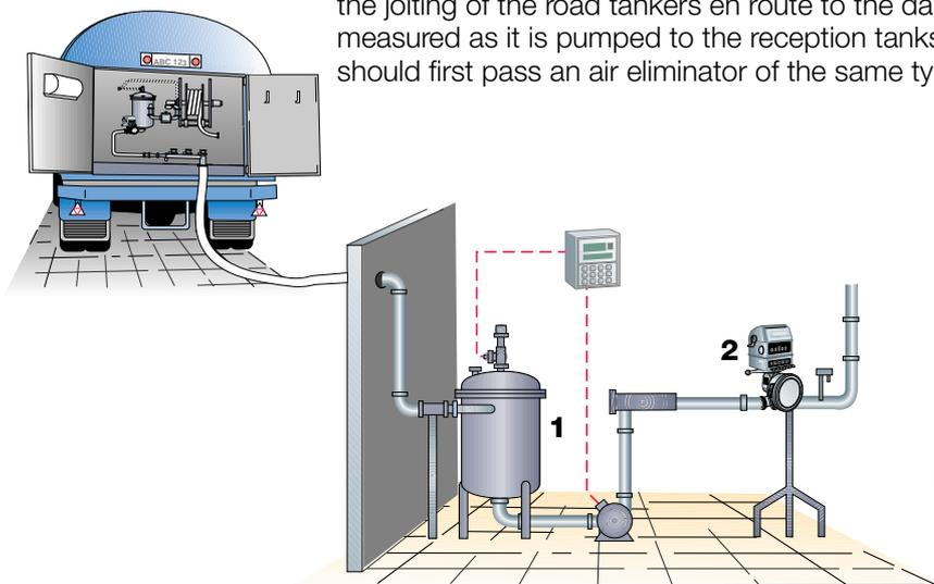
**Fig. 6.6.3** Milk reception at the dairy with air eliminator (1) and volume measuring device (2).
