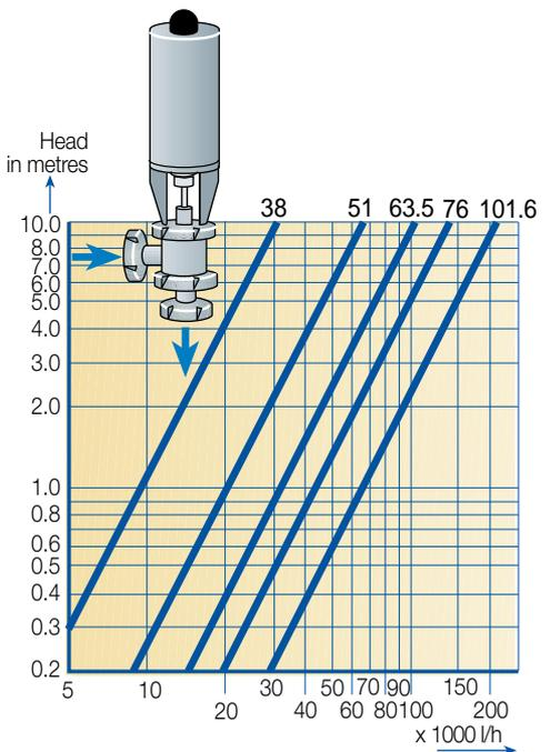
**Fig. 7.11** Pressure-drop graph for a shut-off valve.
