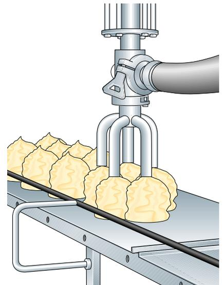
**Fig. 19.5** An extruder in a tray tunnel.
