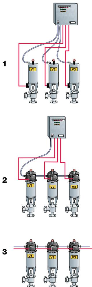
**Fig. 6.8.15** Valve position indication systems.
