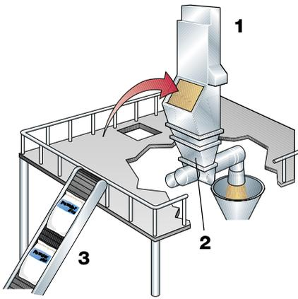
**Fig. 18.1** Equipment for handling powder in sacks.
