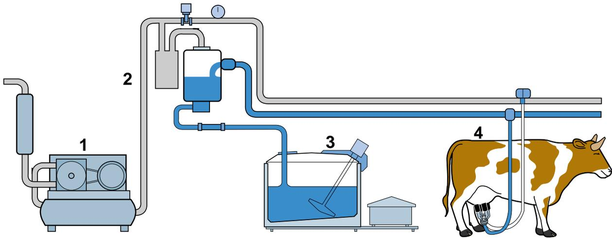
**Fig. 1.8** General design of pipeline milking system.
