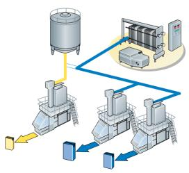
Fig. 9.28 Aseptic tank used as an intermediate storage tank for one product while a second product is processed and packed.
