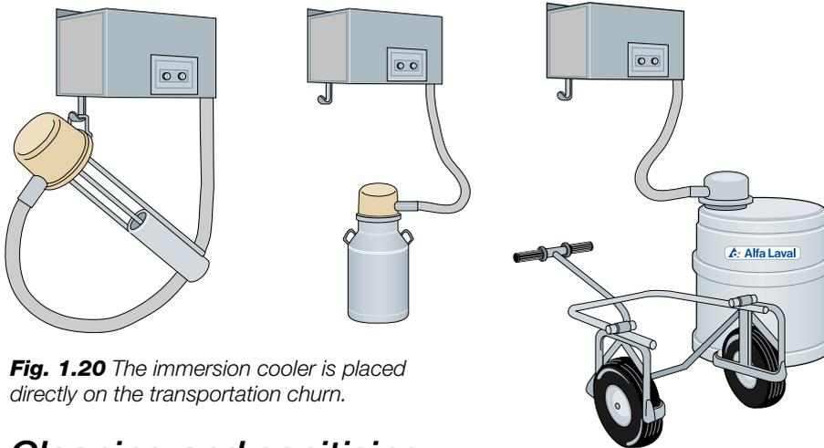
**Fig. 1.20** The immersion cooler is placed directly on the transportation churn.
