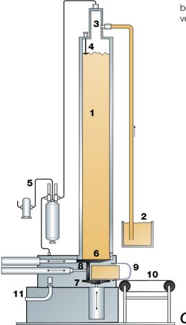
**Fig. 14.24** Block former system for Cheddar-type cheese. Principle and exterior (right).
