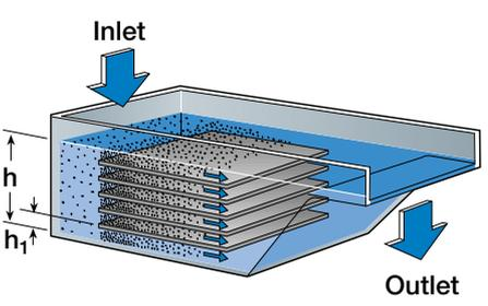
**Fig. 6.2.9** Horizontal baffle plates in the separation vessel increase sedimentation capacity.
