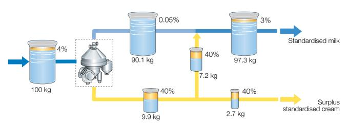
Fig. 6.2.32 Principle of fat standardisation.
