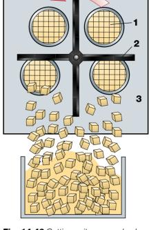
Fig. 14.46 Cutting unit on a curdmaking machine.
