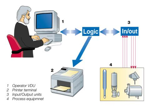
Fig. 6.10.9 Principle of a process control system.
