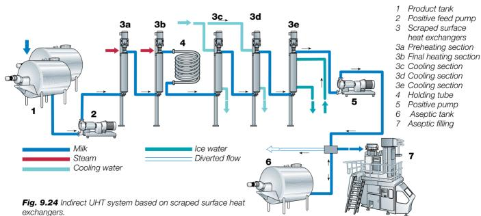
Finally, the cooled product is pumped to an aseptic buffer tank (6) which provides a buffer volume between the continuous process line and the packaging system.
