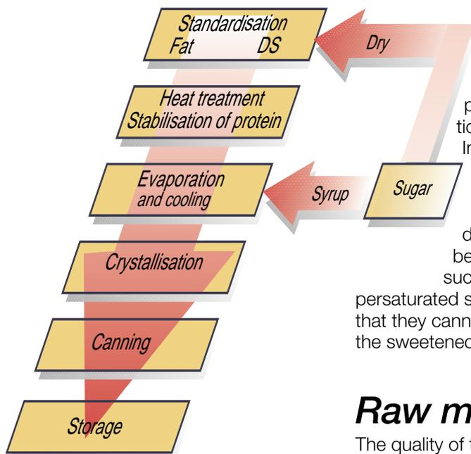
**Fig. 16.2** Process steps for sweetened condensed milk.
