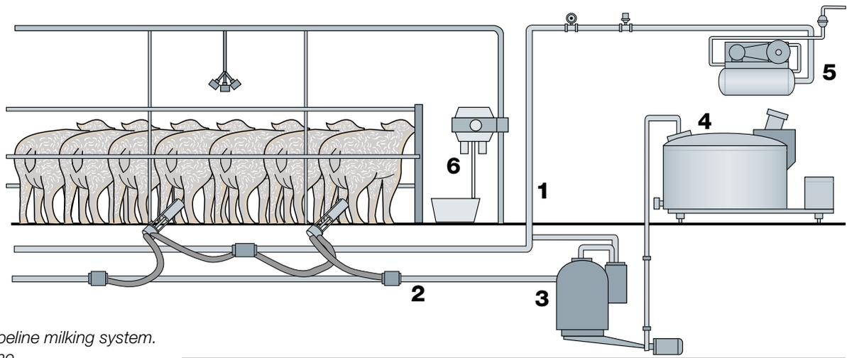
**Fig. 1.17** Pipeline milking system.
