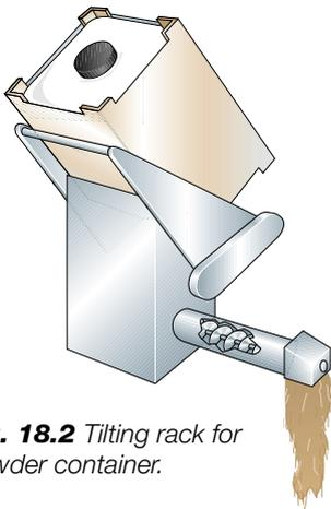
**Fig. 18.2** Tilting rack for powder container.
