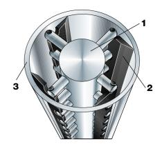
Fig. 6.1.21 Section through a scrapedsurface heat exchanger.
