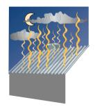
**Fig. 6.1.5** Heat transfer by radiation. Example: A roof accumulates solar heat during the day and radiates the heat at night.
