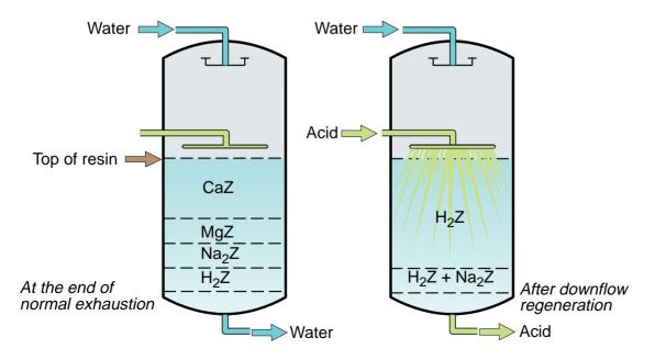
Fig. 15.10 Cation exchanger resin bed before and after regeneration with acid.
