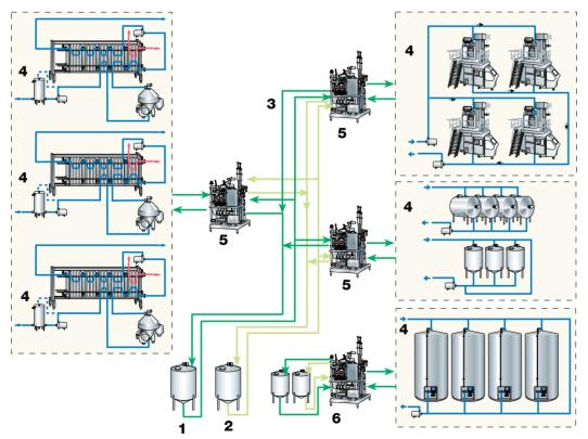
Fig. 21.7 Satellite CIP system
