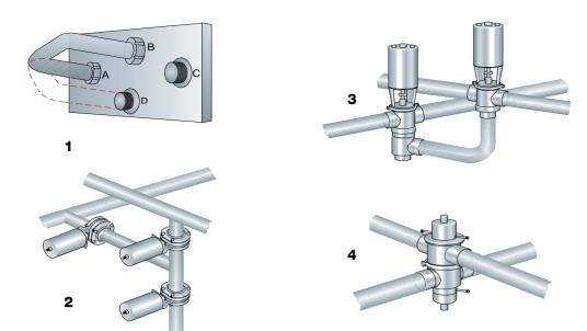
Fig. 6.8.5 Sanitary mixproof valve systems.
