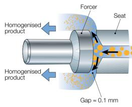
Fig. 6.3.2 At homogenisation the milk is forced through a narrow gap where the fat globules are split.
