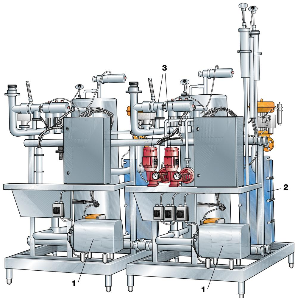
**Fig. 21.8** CIP unit for a decentralised system with two cleaning lines and equipped with two circulation tanks and two dosing pumps for concentrated detergents connected to the detergent and rinse water recovery tanks.
