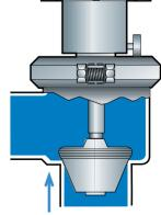
Fig. 6.8.18 Manual control valve with variable-flow plug.
