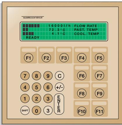
**Fig. 6.10.8** A local operator unit for a pasteuriser.
