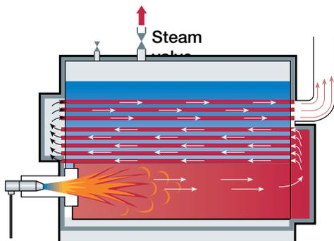
**Fig. 6.11.5** Principle of the fire tube boiler
