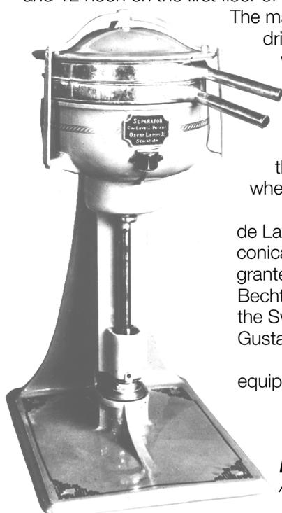
**Fig 6.2.2** One of the very first separators, the Alfa A 1, manufactured from 1882.
