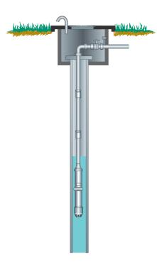
Fig. 6.11.2 Pipe well with submersible pump.
