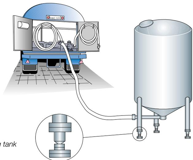
**Fig. 5.13** Milk reception via a weighing tank
