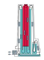
Fig. 9.7 Vertical or tower steriliser.
