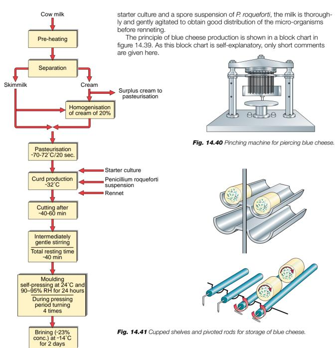
The cheese is pierced after about 5 days in the ripening store to facilitate admission of the oxygen needed for the growth of the mould. Piercing is done with a tool with needles about 2 mm in diameter and roughly equal in length to the height of the cheese. The number of needles depends on the diameter of the cylindrical cheese, which is often pierced alternately through the top and bottom to avoid the risk of its cracking. A piercing machine is shown in figure 14.40.
