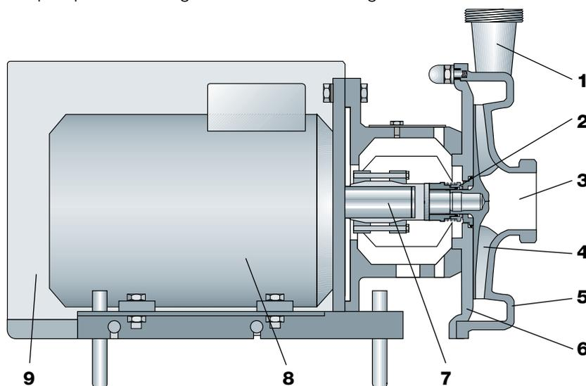
**Fig. 6.7.2** Main parts of a centrifugal pump.
