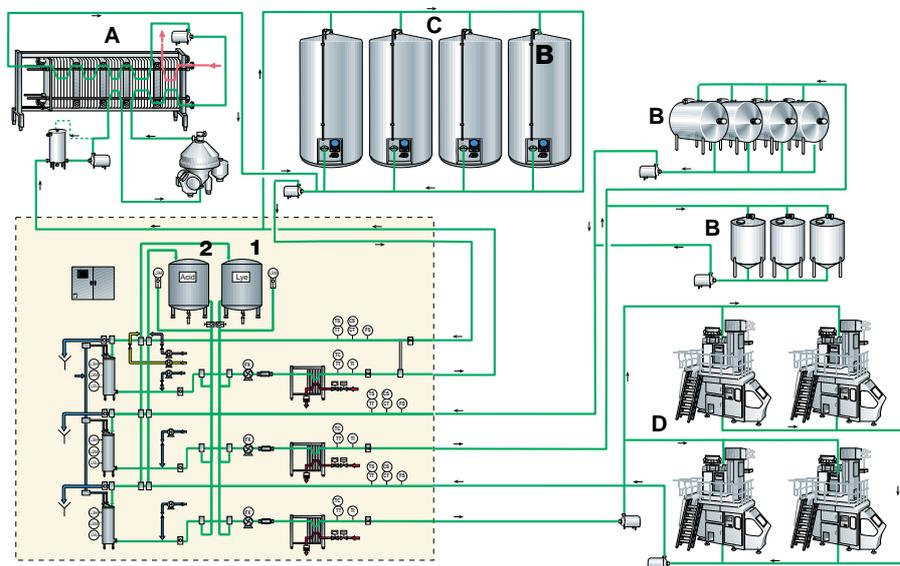
**Fig. 21.5** Principle of the centralised CIP system.
