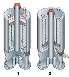
**Fig. 6.8.8** Examples of pneumatically operated actuators.
