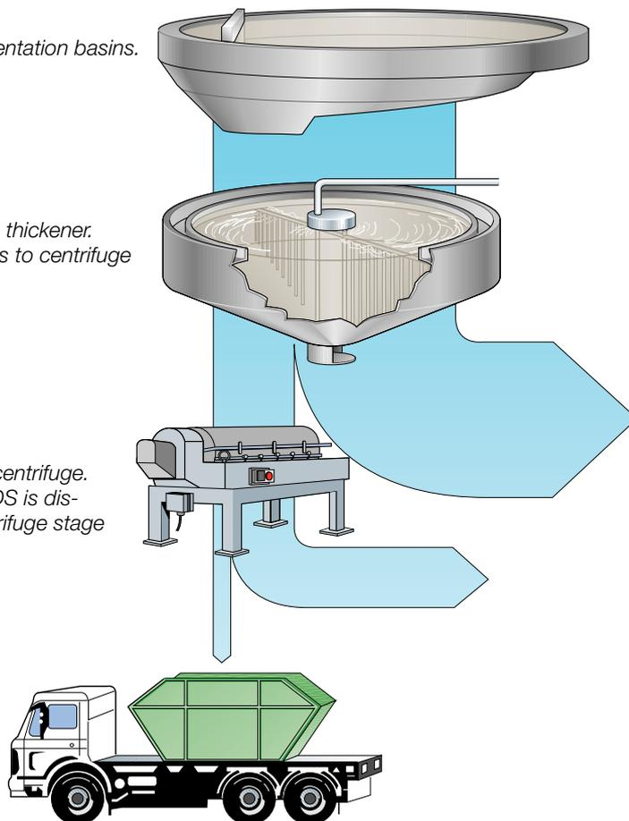
**Fig. 22.5** Reduction in volume of wet sludge from the primary settling stage after treatment in a sludge thickener and decanter centrifuge. The amount of dewatered sludge discharged from the decanter centrifuge is only 8% of the volume of the wet sludge from the sedimentation basins.
