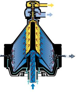
**Fig. 6.2.22** Solids ejection by short opening of the sedimentation space at the periphery of the bowl.
