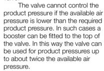
Valves for constant inlet pressure are often used after separators and pasteurisers. Those for constant outlet pressure are used before filling machines.
