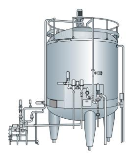
Fig. 18.8 An aseptic tank eleminates the risk of reinfection.
