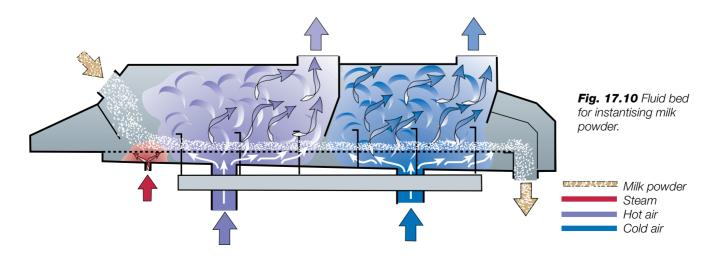
where it is humidified by steam. The vibrations convey the powder through the drying sections, where air at a gradually decreasing temperature is admitted through the powder bed. Agglomeration takes place in the first stage of drying when the particles adhere to each other. Water is evaporated from the agglomerates during their passage through the drying sections. They will have attained the required dryness when they have passed through the fluid-bed casing.
