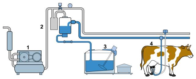
Fig. 1.8 General design of pipeline milking system.
