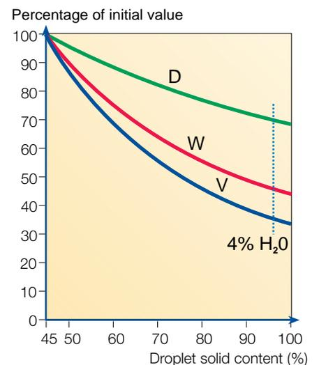
**Fig. 17.4** Weight, volume and diameter decrease of droplet under ideal drying conditions down to 4% H<sub>2</sub>O.
