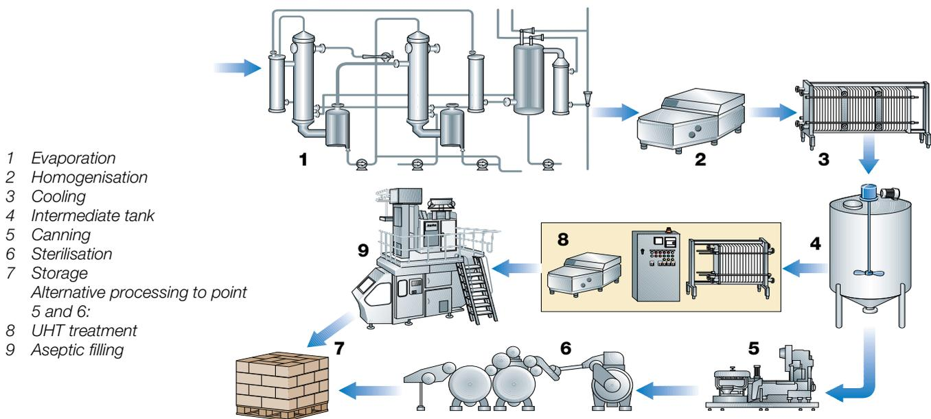
**Fig. 16.3** Process line for unsweetened condensed milk.
