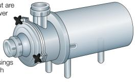
Fig. 6.7.10 Liquid-ring pump.
