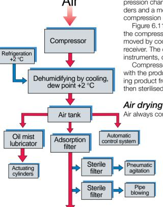
Fig. 6.11.16 Compressed-air installation
