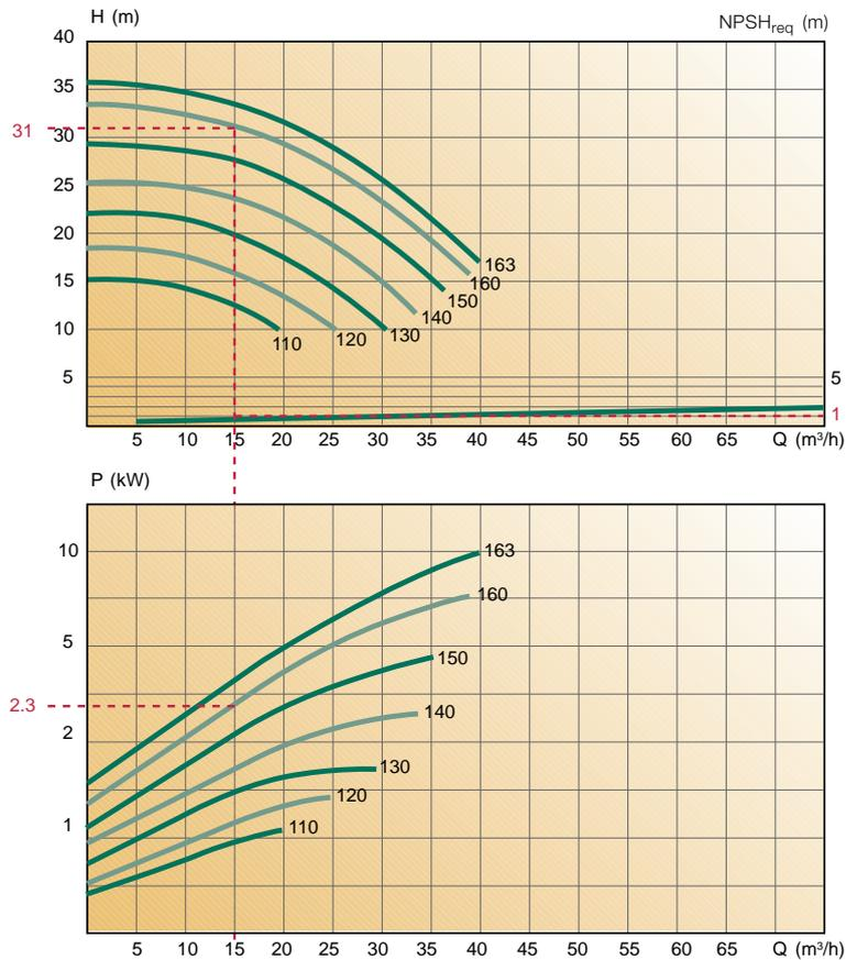
Fig. 6.7.3 Pump chart for a centrifugal pump.
