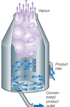
Fig. 6.5.3 Product flow in a vacuum chamber.
