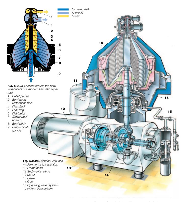
pressure means that the liquid level in the bowl moves inwards. In this way the effects of throttling at the outlets are automatically counteracted. In order to prevent aeration of the product it is important that the paring discs are sufficiently covered with liquid.
