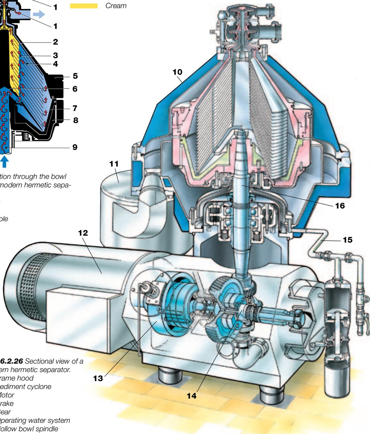
**Fig. 6.2.26** Sectional view of a modern hermetic separator.
