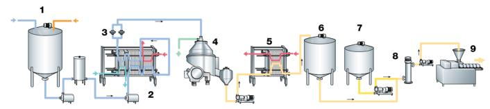
Fig. 14.44 Flowchart for mechanised production of Quarg
