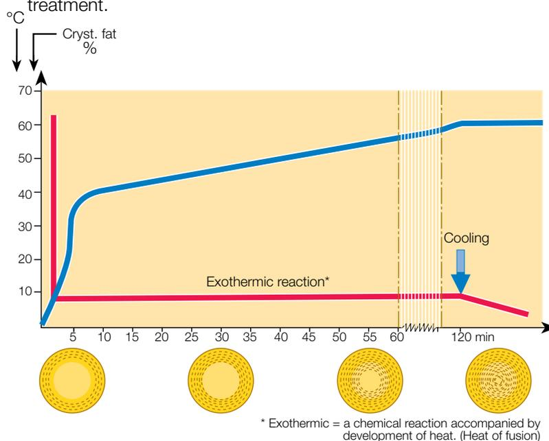
**Fig 2.22** Milk fat crystallisation is an exothermic reaction, which means that the chemical reaction is accompanied by evolution of heat. The crystallisation curve is based on analysis made by the NMR method.
