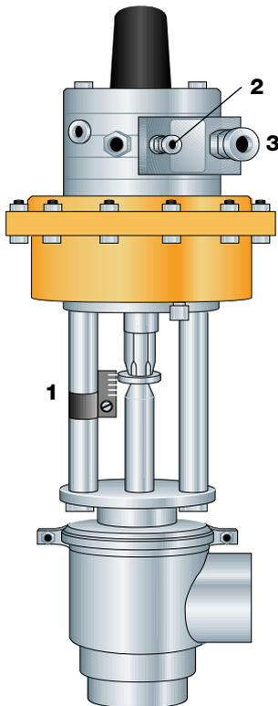
**Fig. 7.16** Pneumatic regulating valve.
