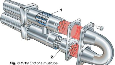
Fig. 6.1.19 End of a multitube tubular heat exchanger.
