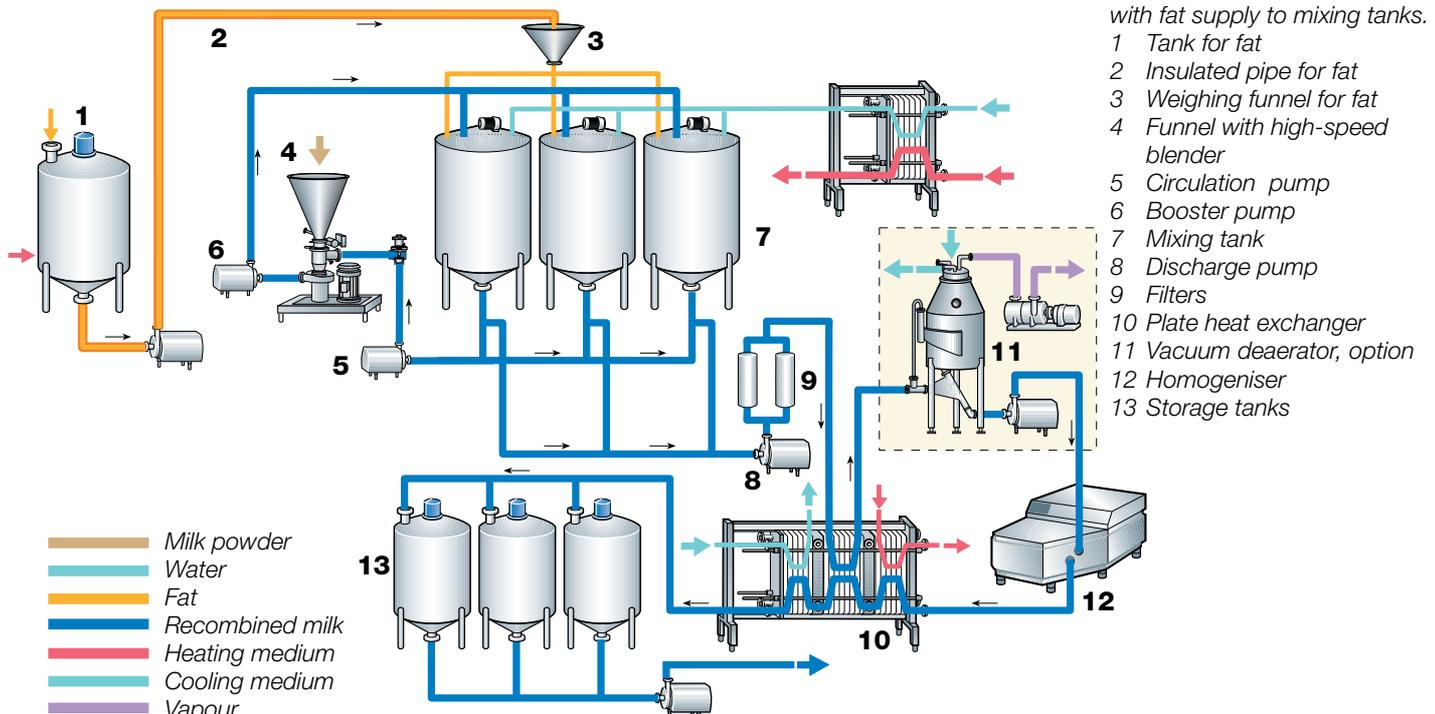
**Fig. 18.5** Recombination plant with fat supply to mixing tanks.
