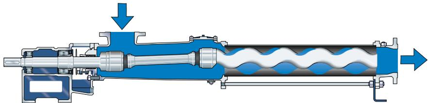
**Fig. 6.7.14** The eccentric-screw pump.
