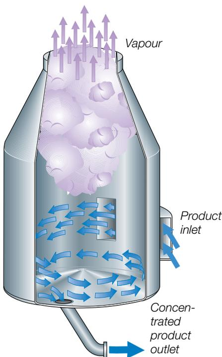
**Fig. 6.5.3** Product flow in a vacuum chamber.
