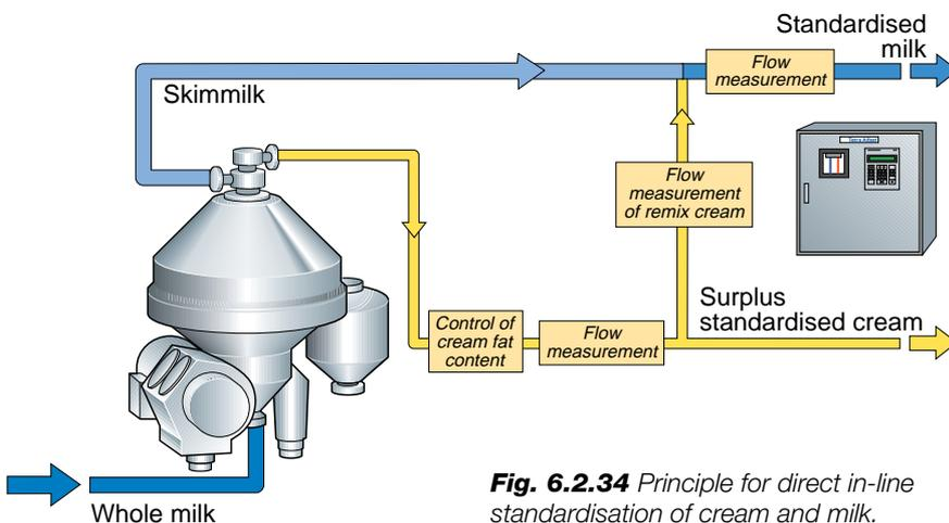
**Fig. 6.2.34** Principle for direct in-line standardisation of cream and milk.
