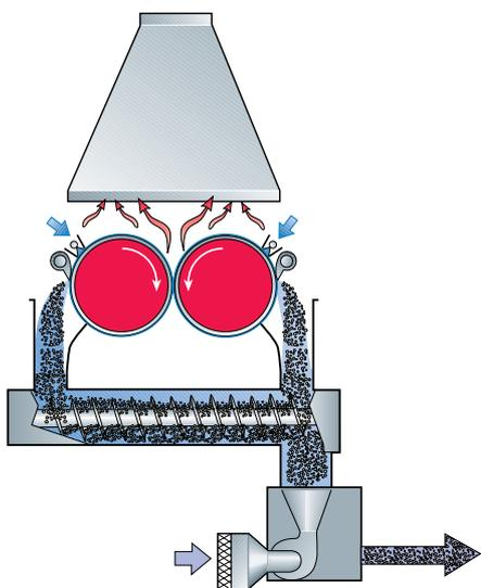
**Fig. 17.2** Principle of the spray-fed roller dryer.
