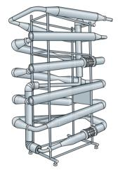
Fig. 20.3 Continuous coagulation, cooking, and syneresis unit for lactic acid, acid and rennet caseins (Pillet).
