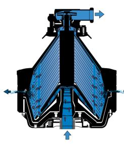
**Fig. 6.2.44** Bowl of one-phase Bactofuge for intermittent discharge of bactofugate.
