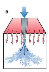
**Fig. 17.5** Stationary nozzles for atomising the milk in a spray drying chamber.
