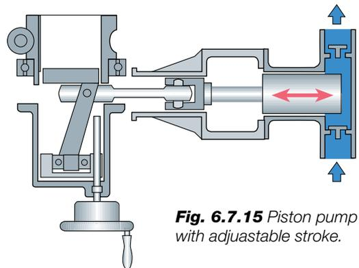
**Fig. 6.7.15** Piston pump with adjustable stroke.
