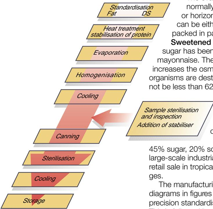
**Fig. 16.1** Process steps for unsweetened condensed milk.
