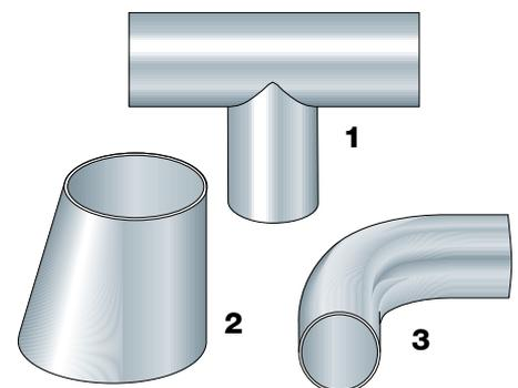
**Fig. 6.8.1** Some examples of fittings for permanent welding.
