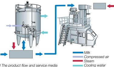
**Fig. 9.26** The product flow and service media connections in an aseptic tank system.
