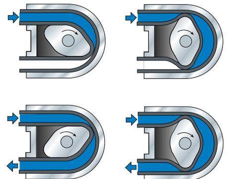
**Fig. 6.7.17** Pumping sequence of a peristaltic pump.
