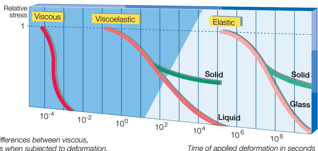
**Fig. 3.1** Curves showing the differences between viscous, viscoelastic and elastic materials when subjected to deformation.
