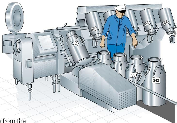
**Fig. 5.9** Churn reception. Weighing and recording of milk.
