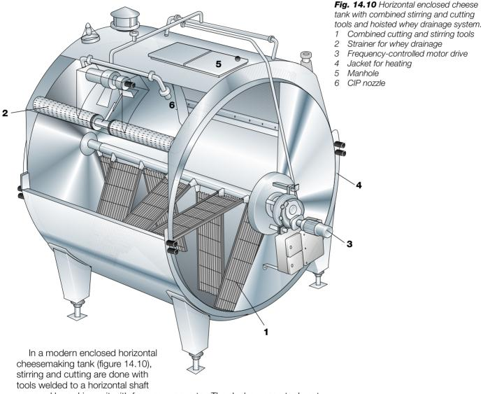
powered by a drive unit with frequency converter. The dual-purpose tools cut or stir depending on the direction of rotation; the coagulum is cut by razor-sharp radial stainless steel knives with the heels rounded to give gentle and effective mixing of the curd.
