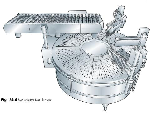
Figure 19.6 shows a type of moulded stick novelty freezer for manufacturing ice cream and water ice bars. The cutaway
