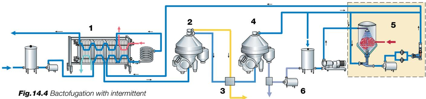
**Fig. 14.4** Bactofugation with intermittent discharge of the bactofugate and optional steriliser.
