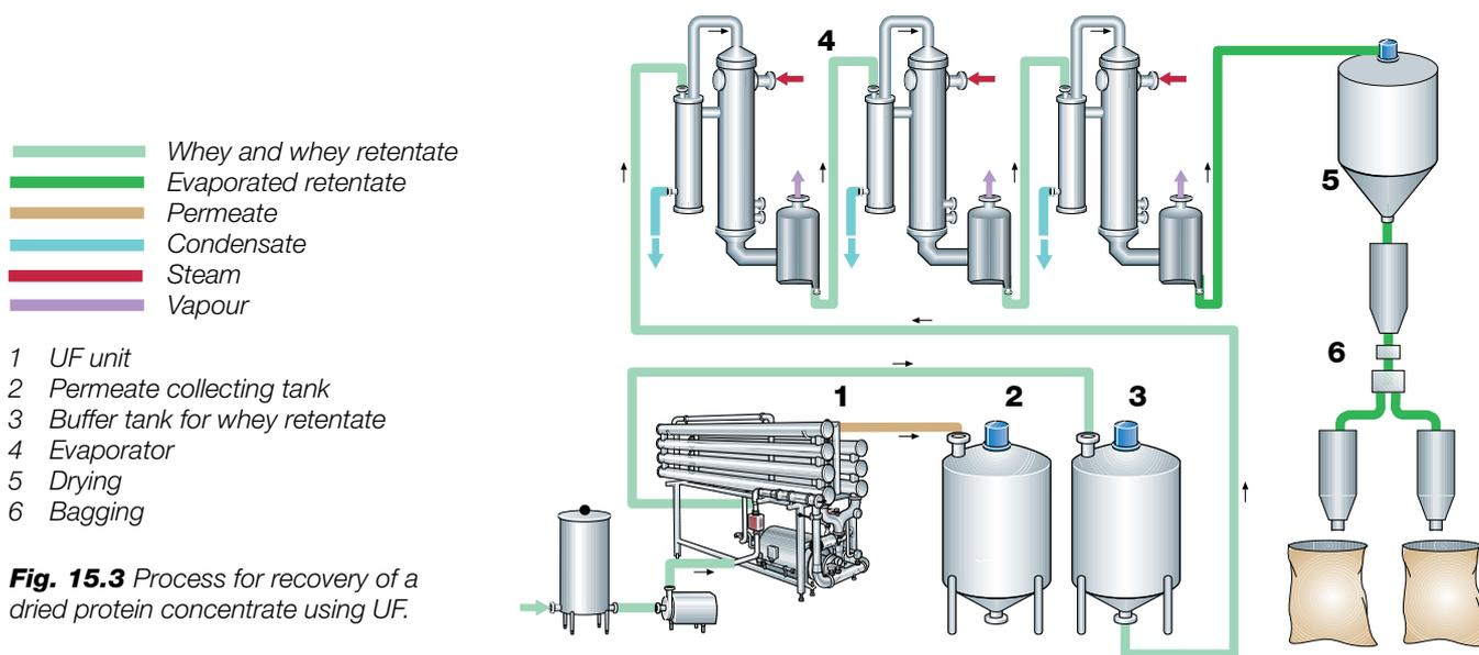
**Fig. 15.3** Process for recovery of a dried protein concentrate using UF.
