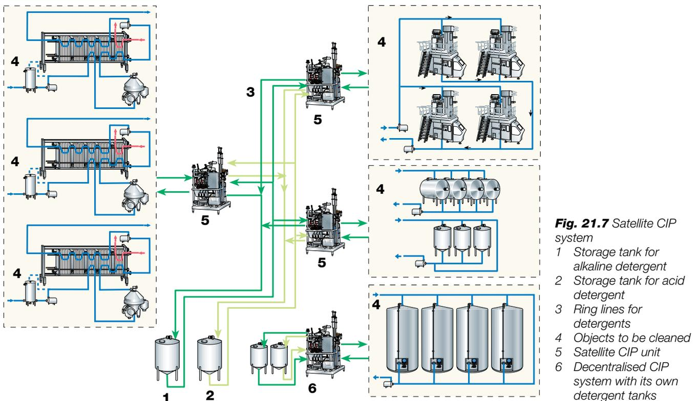
**Fig. 21.7** Satellite CIP system
