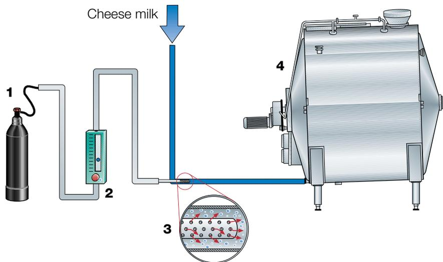
The addition is made in-line in conjunction with filling of the cheesemaking vat/tank as shown in figure 14.8. The rate at which the CO<sub>2</sub> gas is injected, and the time of contact with the milk before rennet admixture, must be calculated when the system is installed. Producers who use carbon dioxide admixture have reported that rennet consumption can be halved with no adverse effects.
