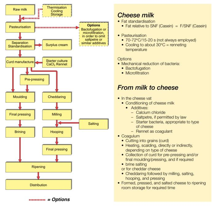
Fig. 14.1 Process flow in production of hard and semi-hard cheese.
