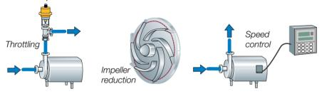
Fig. 6.7.7 Methods of flow control of centrifugal pump.
