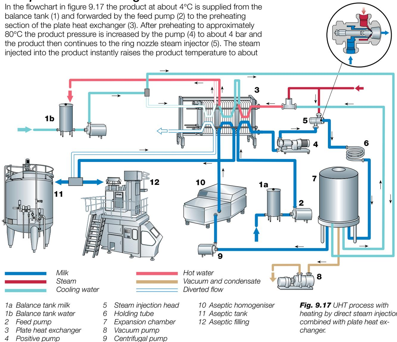
**Fig. 9.17** UHT process with heating by direct steam injection combined with plate heat exchanger.
