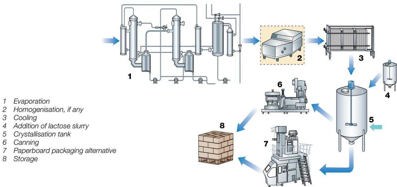
**Fig. 16.4** Process line for sweetened condensed milk.
