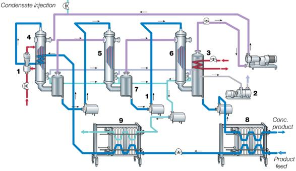
Fig. 6.5.8 Three-effect evaporator with mechanical vapour compression.
