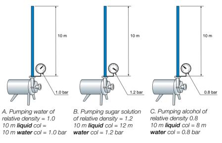
Fig. 6.7.9 Comparison of liquid and water columns for products with different densities.
