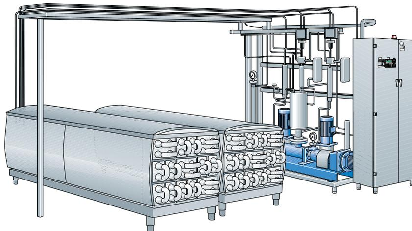
**Fig. 9.30** UHT pilot plant based on tubular heat exchangers.
