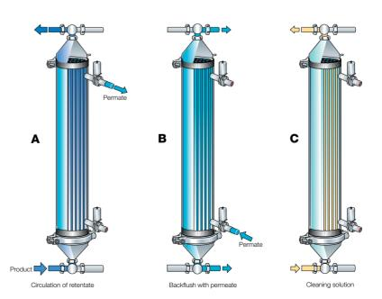
**Fig. 6.4.14** UF cartridge during filtration (A), backflushing (B) and cleaning (C).
