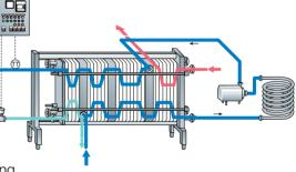
Fig. 7.4 Cooling system for pasteuriser.
