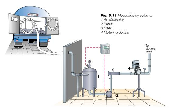
The tanker outlet valve is connected to an air eliminator and from this the milk - free from air - is pumped through the flowmeter, which continuously indicates the total flow. When all the milk has been delivered, a card is placed in the meter for recording the total volume.
