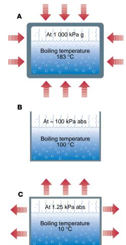
**Fig. 6.11.8** Reduction of pressure causes water to boil at lower temperatures. (g = gauge)
