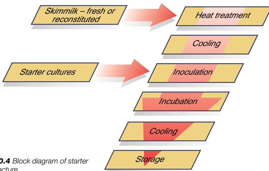
**Fig. 10.4** Block diagram of starter manufacture.
