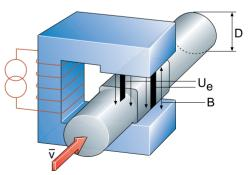
Fig. 6.2.38 Flow transmitter.
