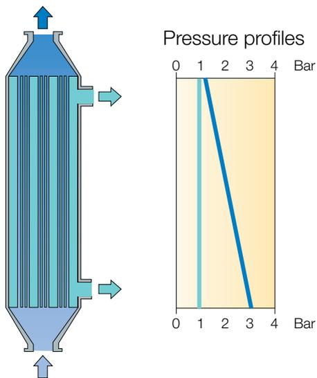
**Fig 6.4.8** Pressure drop during conventional cross-flow microfiltration.
