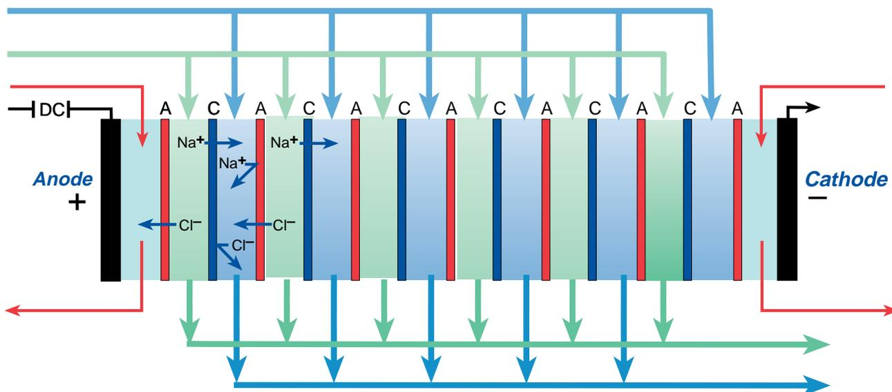
**Fig. 15.9** Cell packs for electrodedialysis.
