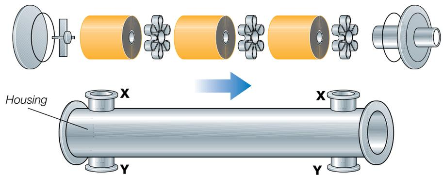
**Fig. 6.4.13** Spiral-wound module assembly. Either or both of the pairs of connecting branches (X and Y) can be used for stackable housing, specially used in UF concepts.
