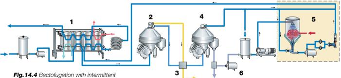
**Fig. 14.4** Bactofugation with intermittent discharge of the bactofugate and optional steriliser.
