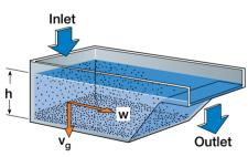
Fig. 6.2.8 Vessel for continuous separation of solids from a liquid.
