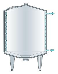
**Fig. 6.9.4** Mixing tank with welded-on heating/cooling channels.
