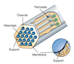
Fig.6.4.6 Cross-flow filtration in a multichannel element (19 channels).
