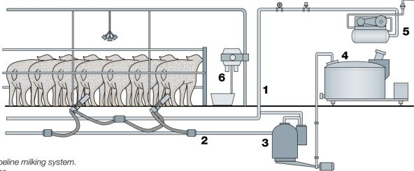
Fig. 1.17 Pipeline milking system.
