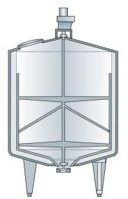
Fig. 6.9.5 An insulated process tank with scraper agitator for viscous products.
