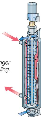
**Fig. 9.16** Scraped surface heat exchanger for heating and cooling.
