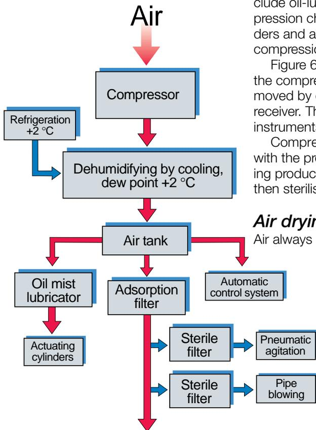
Fig. 6.11.16 Compressed-air installation
