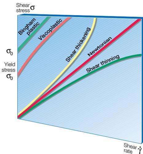
**Fig. 3.4** Flow curves for Newtonian and non-Newtonian fluids.
