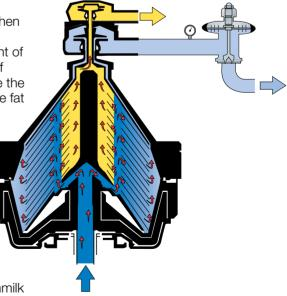
**Fig. 6.2.28** Hermetic separator bowl with an automatic constant pressure unit on the skimmilk outlet.
