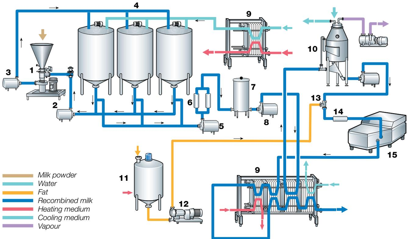
**Fig. 18.7** Recombination plant with in-line fat mixing.
