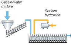
Fig. 20.6 An extrusion cooking system.
