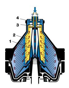
Fig. 6.2.23 Semi-open (paring disc) self-cleaning separator.
