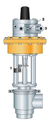
Fig. 7.16 Pneumatic regulating valve.
