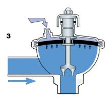
Fig. 6.8.21 Function of the constantpressure valve when regulating the pressure before the valve.
