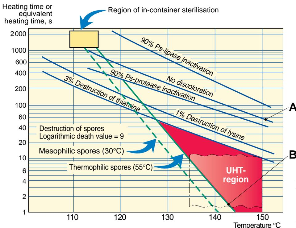
**Fig. 9.5** Limiting lines for destruction of spores and effects on milk. The values within brackets (30°C and 55°C) express the optimal growth temperatures of the vital types of corresponding spore forming micro-organisms. Source: Kessler
