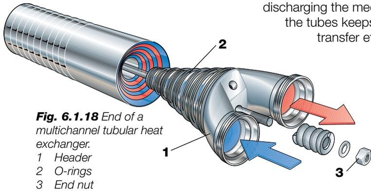
**Fig. 6.1.18** End of a multichannel tubular heat exchanger.
