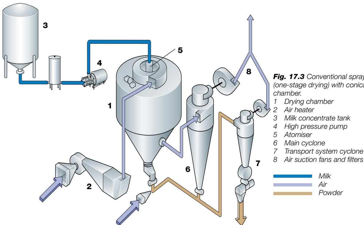
**Fig. 17.3** Conventional spray dryer (one-stage drying) with conical base chamber.
