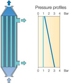
Fig 6.4.8 Pressure drop during conventional cross-flow microfiltration.
