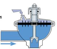
then moves upwards, increasing the passage for the product. The flow will then increase until the product pressure has dropped to the preset value. This valve is available in two versions for constant pressure before or after the valve.
