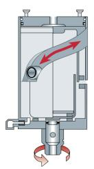
**Fig. 6.8.11** Principle of the air driven actuator for butterfly valves.
