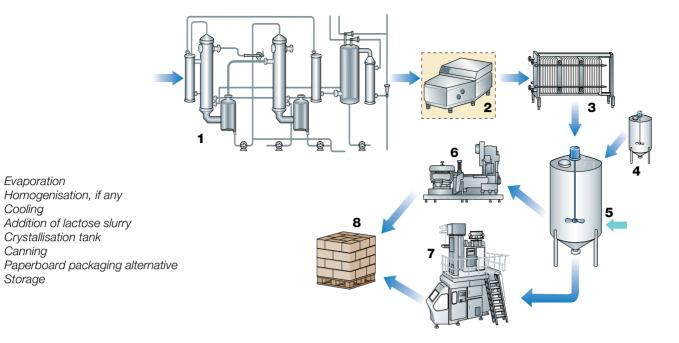
Fig. 16.4 Process line for sweetened condensed milk.
