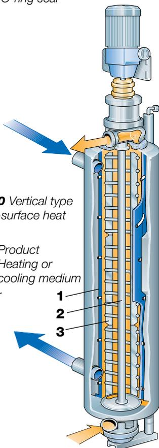
**Fig. 6.1.20** Vertical type of scraped-surface heat exchanger.
