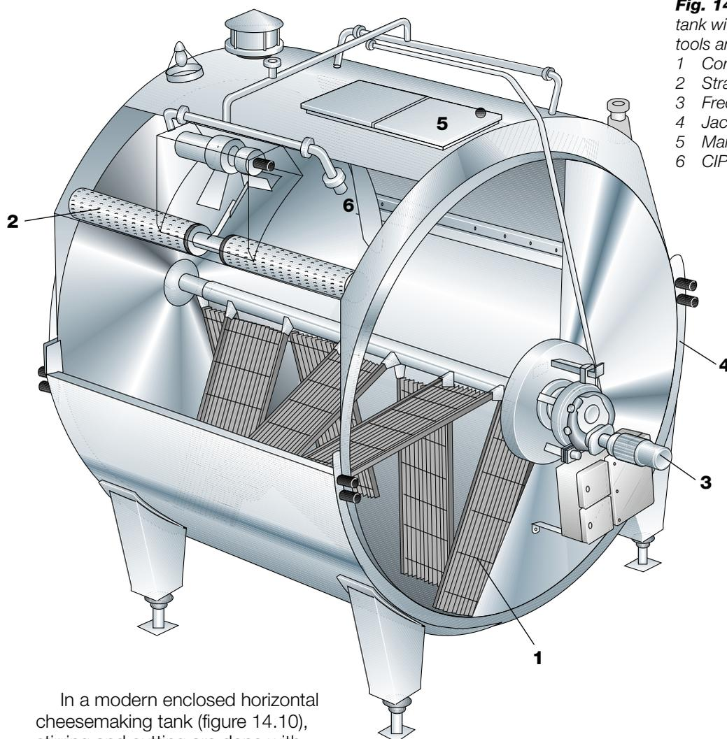
In a modern enclosed horizontal cheesemaking tank (figure 14.10), stirring and cutting are done with tools welded to a horizontal shaft powered by a drive unit with frequency converter. The dual-purpose tools cut or stir depending on the direction of rotation; the coagulum is cut by razor-sharp radial stainless steel knives with the heels rounded to give gentle and effective mixing of the curd.
