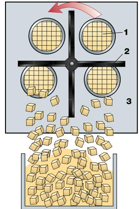
**Fig. 14.46** Cutting unit on a curdmaking machine.
