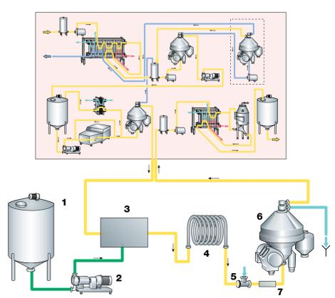
**Fig. 13.5** Neutralisation of free fatty acids (FFA) can be one of the refining processes in the production of Anhydrous Butteroil or Butteroil.
