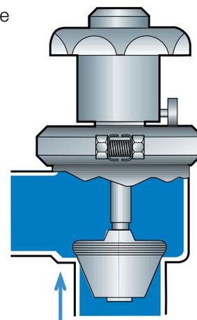
**Fig. 6.8.18** Manual control valve with variable-flow plug.
