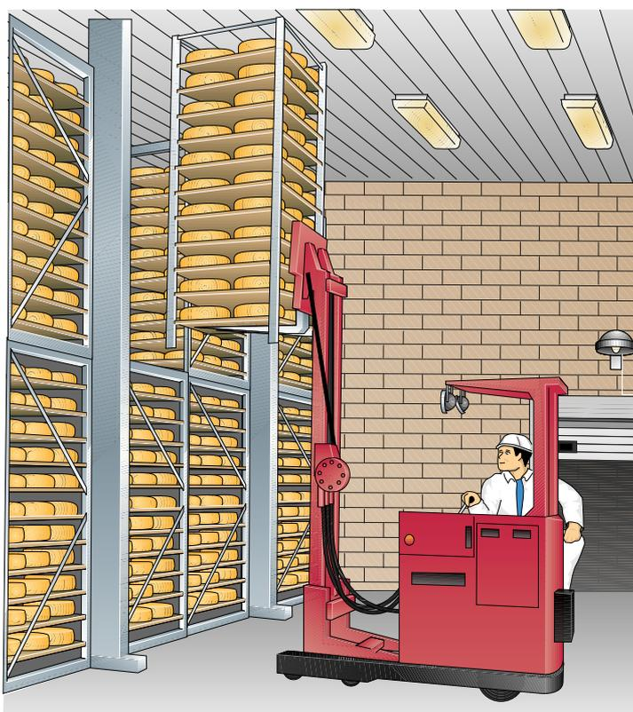
follow at 12 – 18°C and 75 – 80% RH. Finally the cheese is transferred to a storage room at about 10 – 12°C and a relative humidity of about 75%, where the final characteristics are developed.
