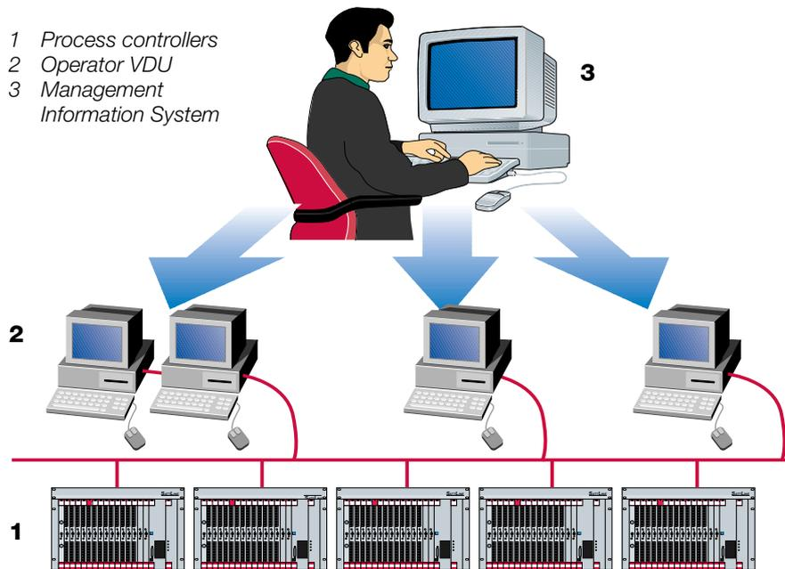
**Fig. 6.10.15** Totally integrated system including Management Information System.
