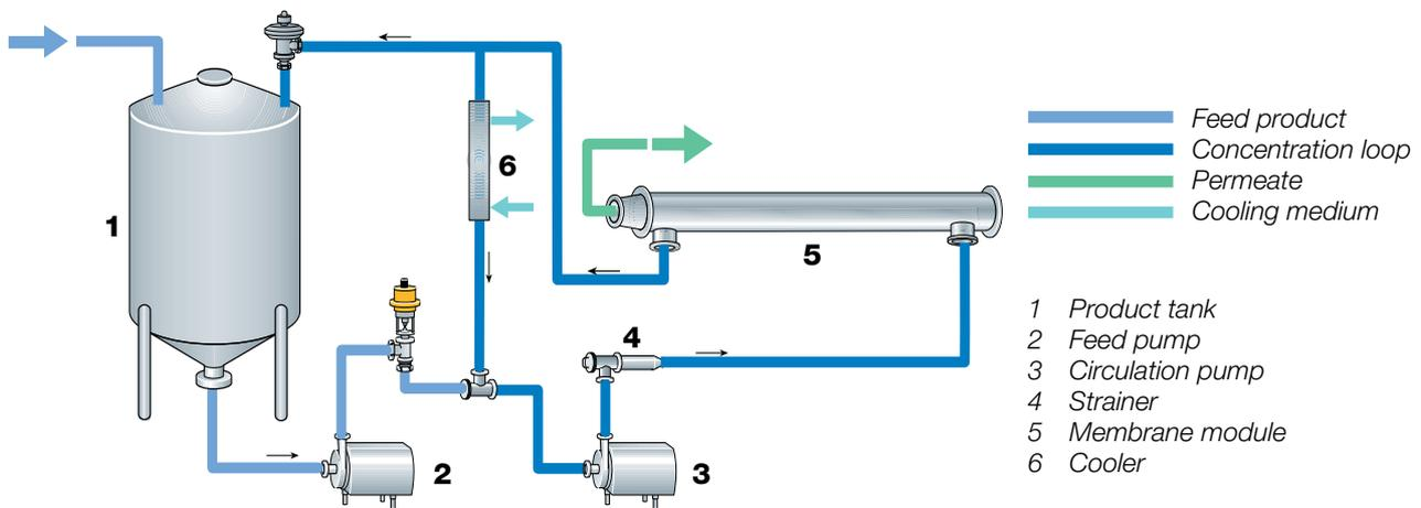
**Fig. 6.4.17** Batch membrane filtration plant
