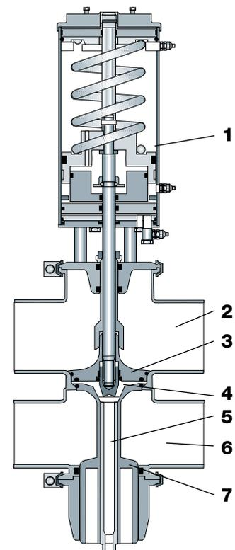
**Fig. 6.8.13** Double-seat mixproof valve with balanced plug and built-in seat lift
