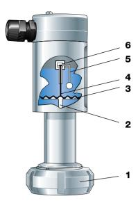
Fig. 7.13 Pressure transmitter
