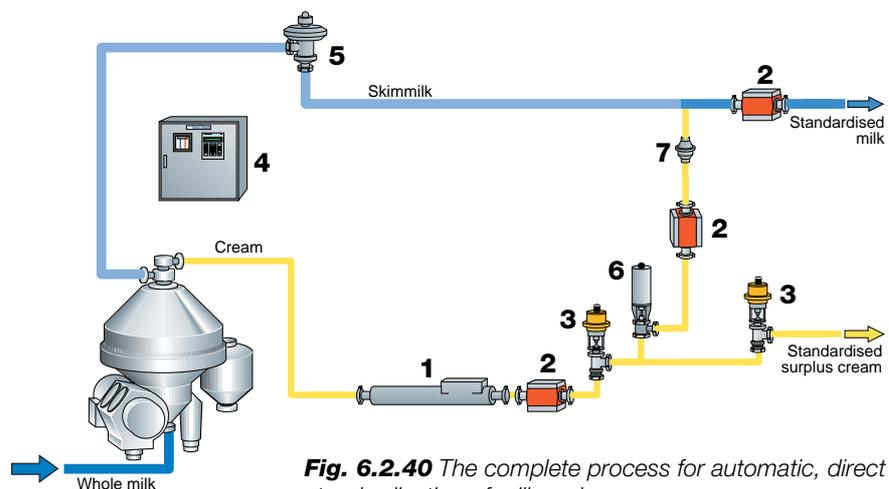
**Fig. 6.2.40** The complete process for automatic, direct standardisation of milk and cream.
