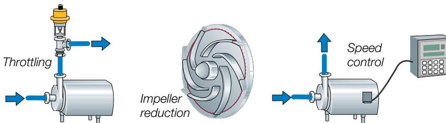
**Fig. 6.7.7** Methods of flow control of centrifugal pump.
