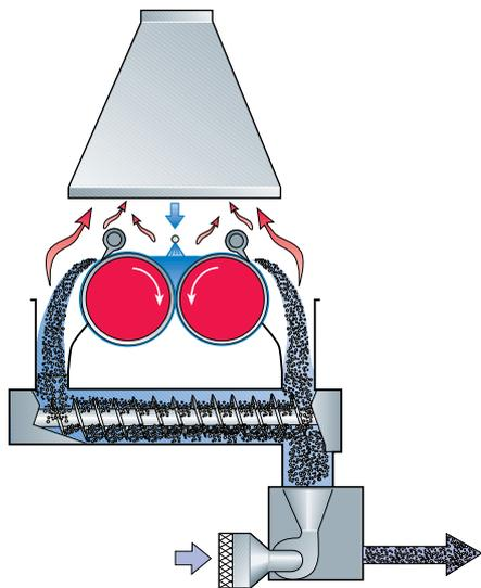
**Fig. 17.1** Principle of the trough-fed roller dryer.
