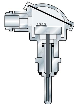
**Fig. 7.14** Resistance type temperature transmitter
