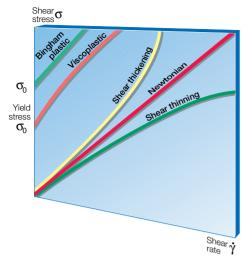
**Fig. 3.4** Flow curves for Newtonian and non-Newtonian fluids.
