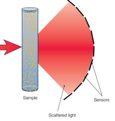
Fig. 6.3.7 Particles analysis by laser diffraction.
