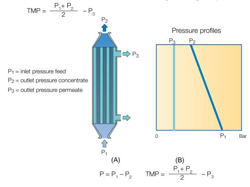
Fig. 6.4.16 Hydraulic (A) and transmembrane (B) pressure drops over a membrane
