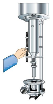
**Fig. 6.1.22** Removal of blades from the rotor assembly in lowered position.
