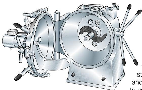
**Fig. 14.49** Cooker, open and tilted for emptying.
