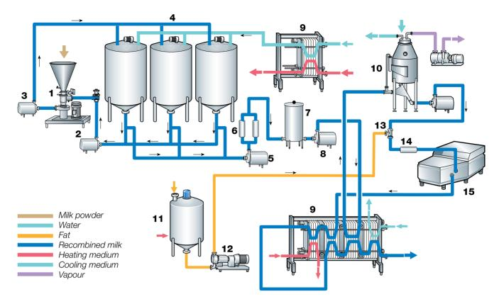
place as described earlier. The milk then flows through an in-line injector (13), where liquid fat from the fat-melting tank (11) is continuously metered into the flow by a positive displacement proportioning pump (12). Blending is completed in an in-line mixer (14) downstream of the injector.
