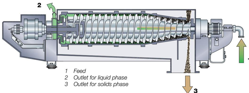
**Fig. 15.8** Decanter centrifuge.
