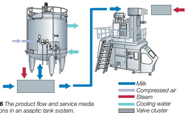
**Fig. 9.26** The product flow and service media connections in an aseptic tank system.
