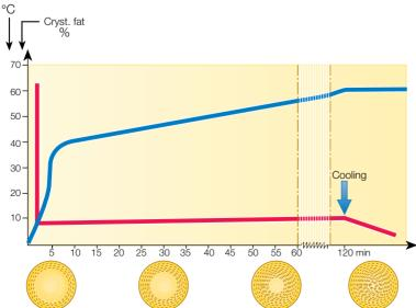
**Fig. 8.4** The crystallisation process for 40% cream at 8%.
