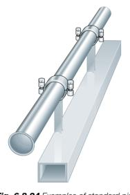
**Fig. 6.8.24** Examples of standard pipe supports.
