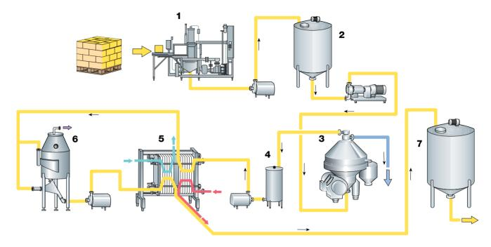
Fig. 13.4 Production line for AMF from butter.
