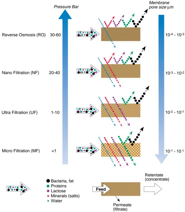
Fig 6.4.3 Principles of membrane filtration.
