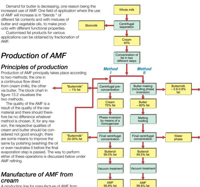
Fig. 13.2 Block chart showing principle of AMF production.
