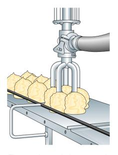
Fig. 19.5 An extruder in a tray tunnel.
