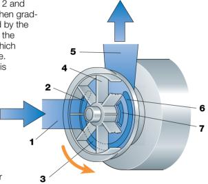
**Fig. 6.7.11** Working principle of a self-priming liquid-ring pump.
