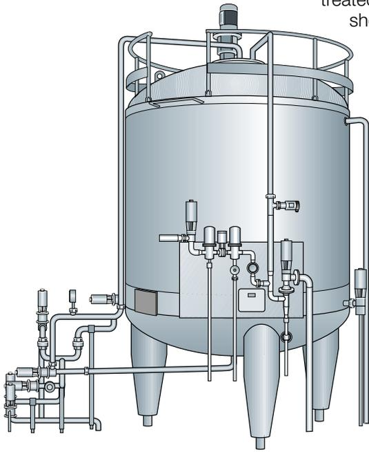
**Fig. 9.25** Aseptic tank with accessories.
