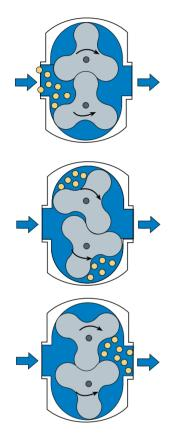
Fig. 6.7.13 Lobe-rotor pump principle.
