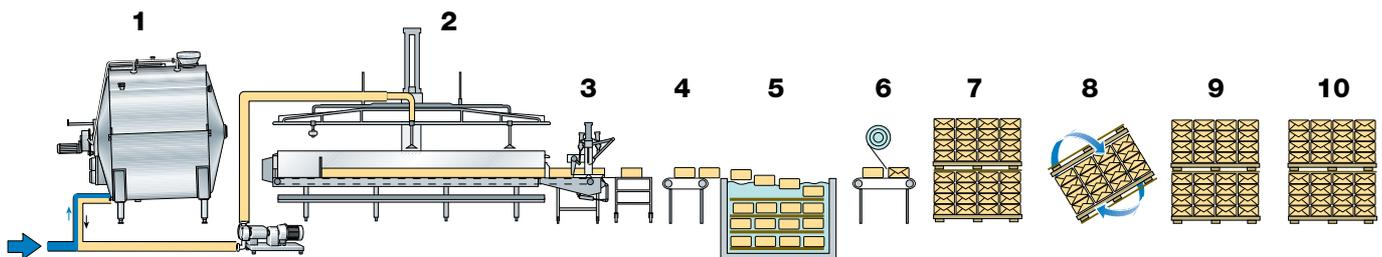
**Fig. 14.34** Flowchart for mechanised production of rindless Emmenthal cheese.
