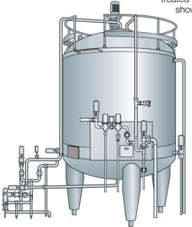
Fig. 9.25 Aseptic tank with accessories.
