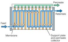
**Fig. 6.4.4** Example of a plate and frame system (DDS) for UF.
