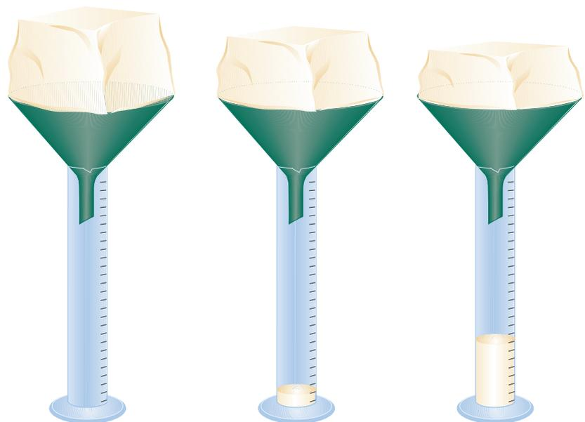
**Fig. 8.3** Test of leakage of whipped cream after 2 hours at 18–20°C and 75% R.H.
