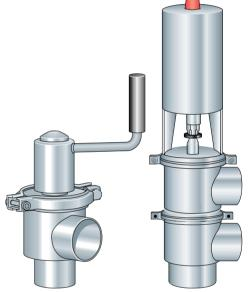
Fig. 6.8.6 Manual shut-off seat valve and pneumatically operated change-over seat valve. The operating mechanism is interchangable between shut-off and change-over seat valves.
