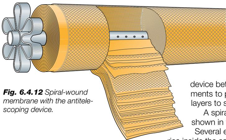
**Fig. 6.4.12** Spiral-wound membrane with the antitelescoping device.
