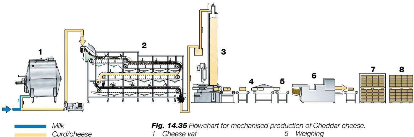
**Fig. 14.35** Flowchart for mechanised production of Cheddar cheese.
