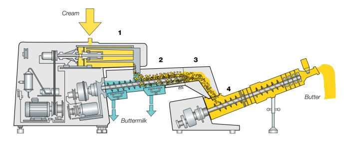
**Fig. 12.6** A continuous buttermaking machine
