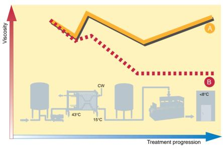
Fig.11.16 Viscosity development of stirred yoghurt during cooling, packing and cold storage.
