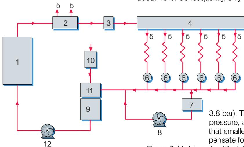
**Fig. 6.11.4** Steam production and distribution system
