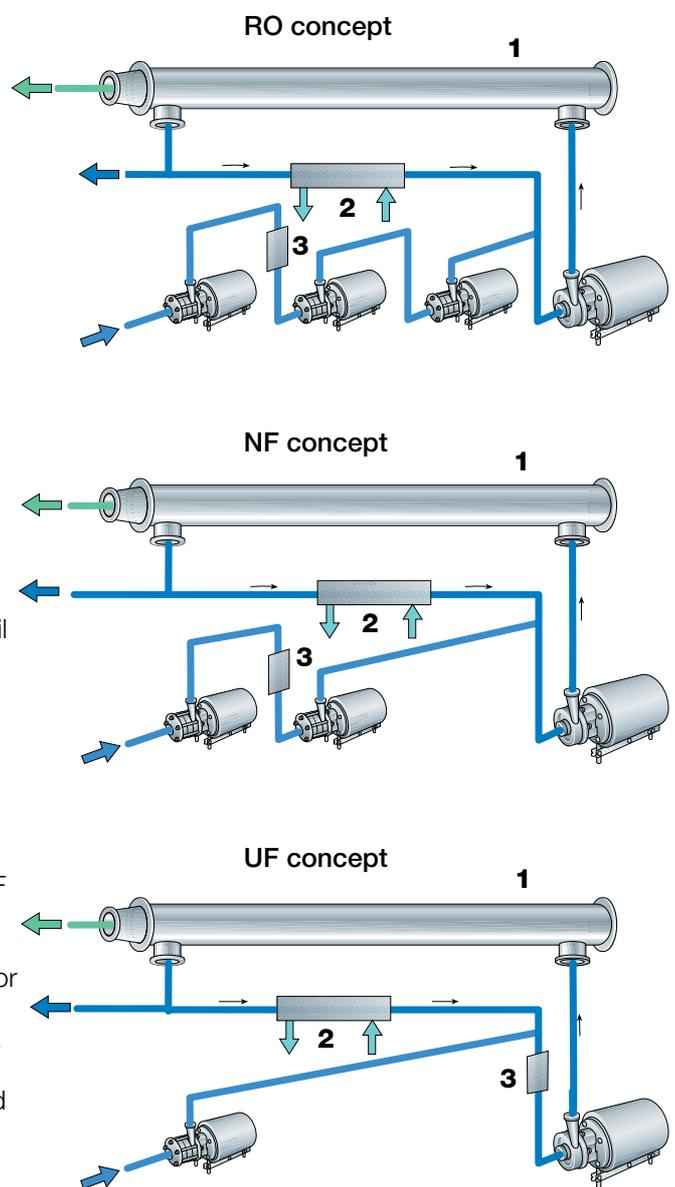
**Fig. 6.4.18** Design principles for different filter loops.
