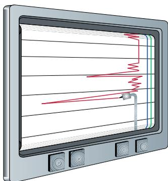
**Fig. 6.10.3** Analog control can be exemplified by the control of the pasteurisation temperature.
