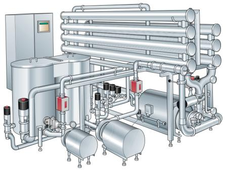
Fig. 6.4.20 Production module for UF processing.
