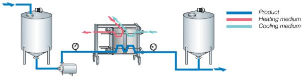
Fig. 7.10 Pressure drop can be shown by pressure guages in the process line.
