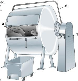
Fig. 12.4 Butter churn for batch production.
