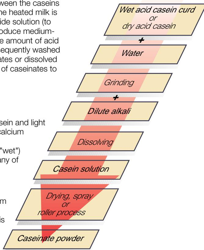
**Fig. 20.5** Basic steps involved in the manufacture of spray or roller dried caseinates from acid casein curd or dry acid casein. Alkali may be sodium hydroxide, potassium hydroxide, calcium hydroxide, or ammonia.
