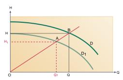
Fig. 6.7.8 Flow reduction when the impeller diameter is reduced from D to D<sub>1</sub>.
