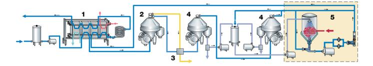
Without any mechanical means of reducing spores it is normal to add some 15-20 g of sodium nitrate per 100 l of milk to inhibit their growth, but with *single* bactofugation and a high load of spores in milk, 2.5-5 g per 100 l of milk will prevent the remaining spores from growing.
