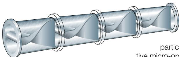
**Fig. 11.15** Fruit mixer built into the pipe.
