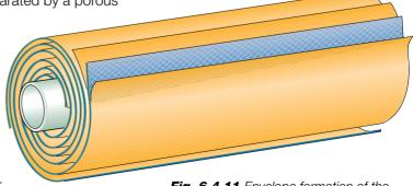
**Fig. 6.4.11** Envelope formation of the spiral-wound filter design.
