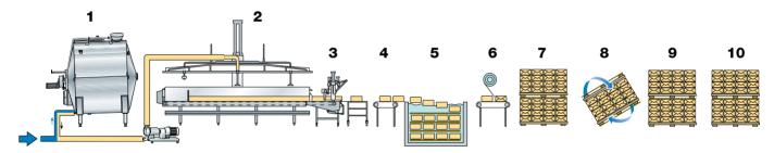
Fig. 14.34 Flowchart for mechanised production of rindless Emmenthal cheese.
