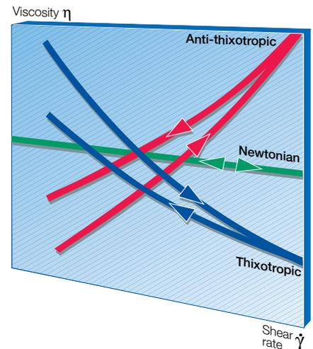
Fig. 3.7 Viscosity curves for time-dependent non-Newtonian fluids.
