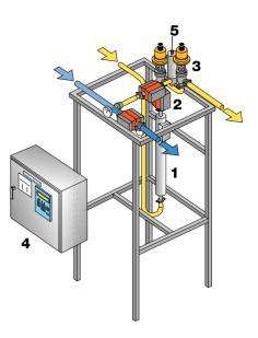
**Fig. 6.2.33** Direct in-line standardisation systems are pre-assembled as process units.
