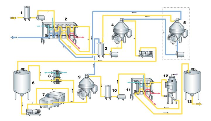
Fig. 13.3 Production line for AMF from cream
