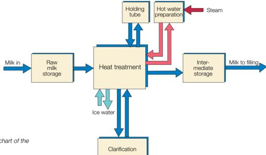
Fig. 7.1 Generalised block chart of the milk pasteurisation process.
