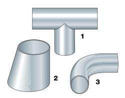
**Fig. 6.8.1** Some examples of fittings for permanent welding.
