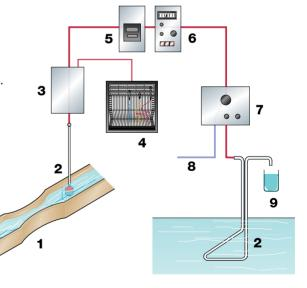
Fig. 22.2 Automatic sampling system.
