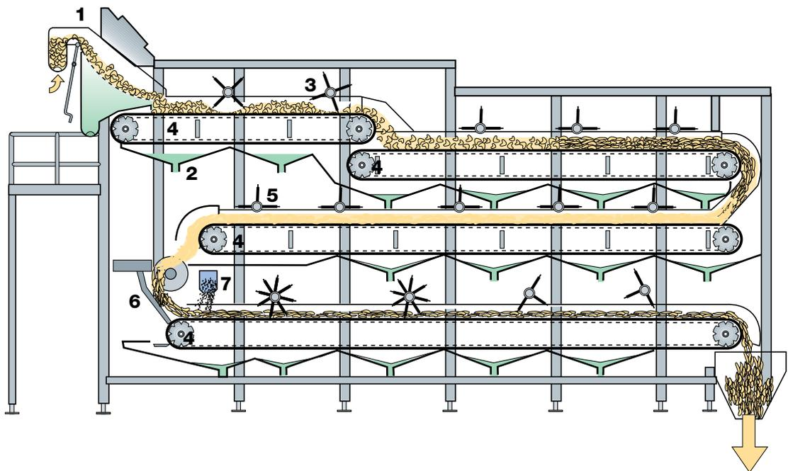
**Fig. 14.20** Continuous system for de-wheying, cheddaring, milling, and salting curd intended for Cheddar cheese.
