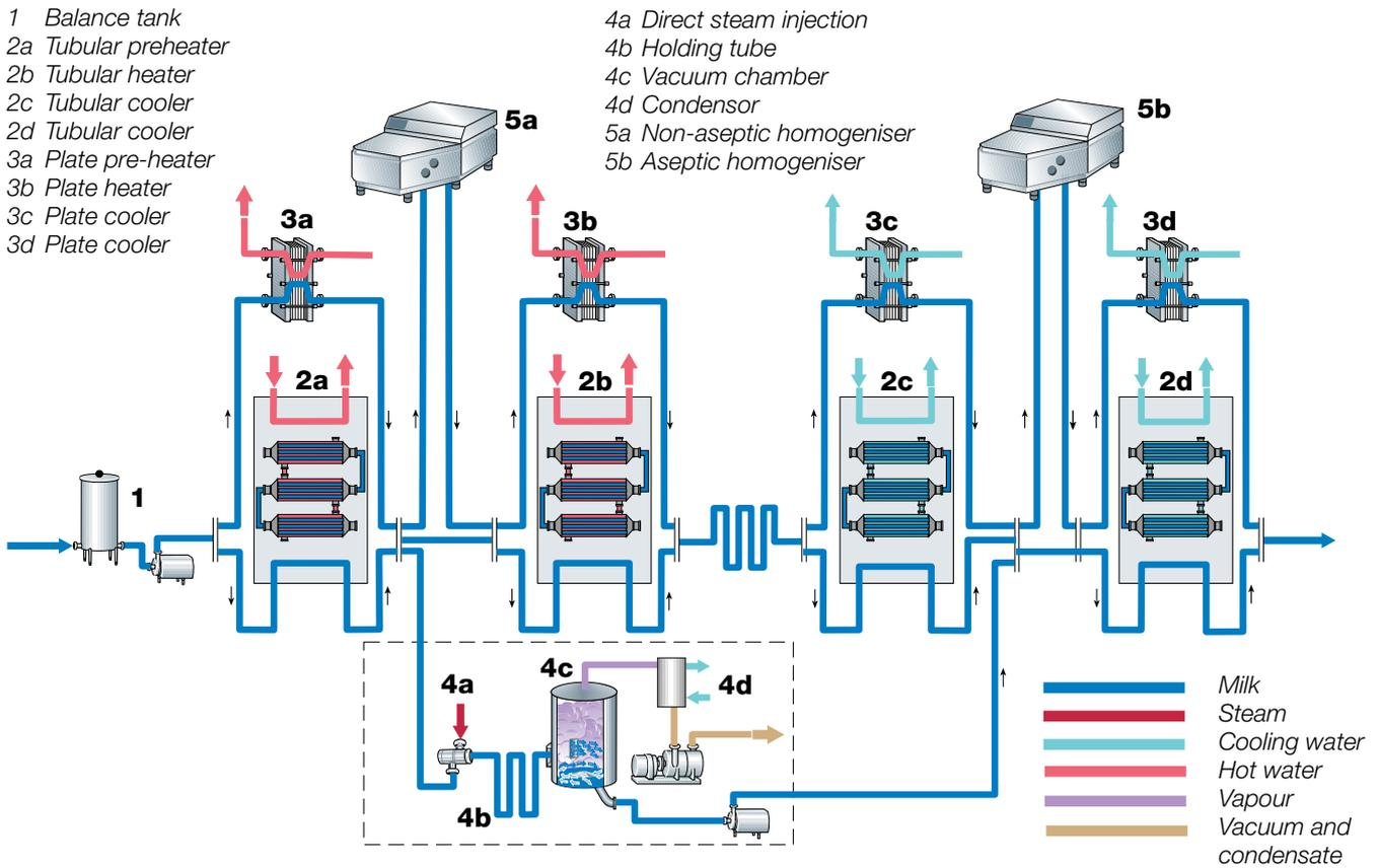
**Fig. 9.31** Process flow chart for UHT pilot plant including indirect heating in plate heat exchangers or tubular heat exchangers and direct heating module (within broken line) as well as aseptic and non-aseptic homogenisation alternatives.
