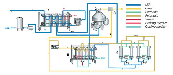
content in the cheese milk, is routed by a standardisation device to the sterilisation plant.
