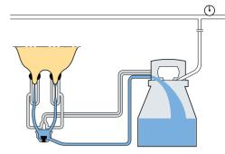
Fig. 1.5 Machine milking equipment.
