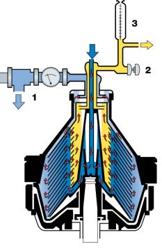
**Fig. 6.2.27** Paring-disc separator with manual control devices in the outlets.
