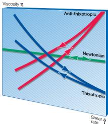
Fig. 3.7 Viscosity curves for timedependant non-Newtonian fluids.
