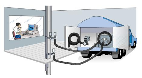
**Fig. 5.10** Measuring milk intake in a tanker reception hall
