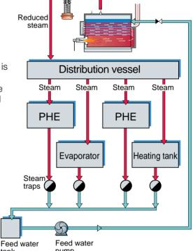
Fig. 6.11.7 System for steam distribution and condensate collection.
