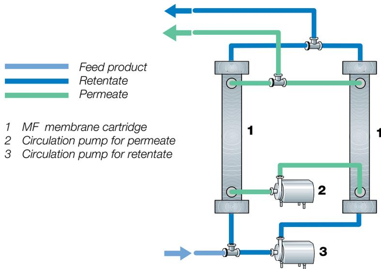
**Fig. 6.4.19** Design principle of a MF filter loop.
