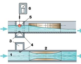
Fig. 22.1 System for measuring the flow in an open canal with a venturi flume.
