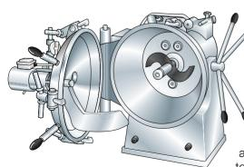
Fig. 14.49 Cooker, open and tilted for emptying.
