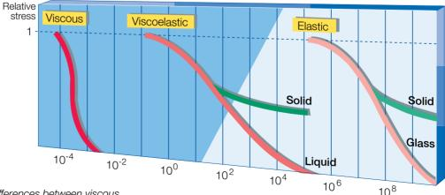
Fig. 3.1 Curves showing the differences between viscous, viscoelastic and elastic materials when subjected to deformation.
