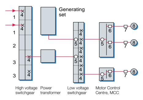
Fig. 6.11.17 Example of a power distribution system for a dairy plant.
