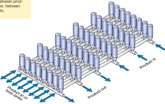
Fig. 6.8.23 Valve arrangement in a tank garden for independent routing of products and cleaning solutions to and from the tanks.
