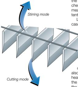
**Fig. 14.11** Cross-section of the combined cutting and stirring tool blade with sharp cutting edge and blunt stirring edge.
