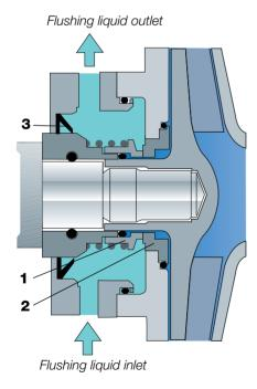
Fig. 6.7.5 Flushed shaft seal
