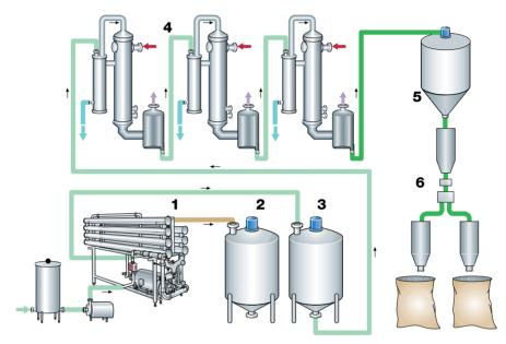
To obtain an 85% protein concentrate the liquid whey is first concentrated 20 – 30-fold by direct ultrafiltration to a solids content of approximatively 25%; this is regarded as the maximum for economic operation. It is then necessary to diafilter the concentrate to remove more of the lactose and
