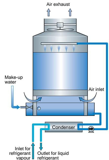
**Fig. 6.11.14** Combined tube condenser and cooling tower circuit.
