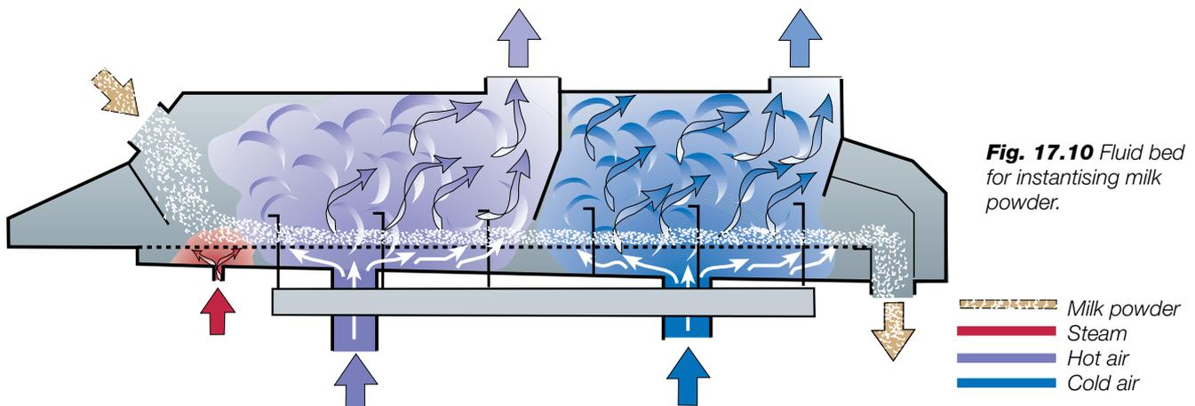
**Fig. 17.10** Fluid bed for instantising milk powder.
