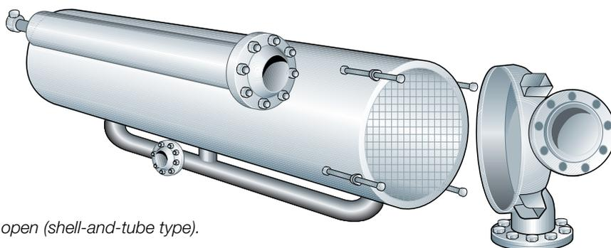
**Fig. 6.11.13** Tube condenser with front end open (shell-and-tube type).
