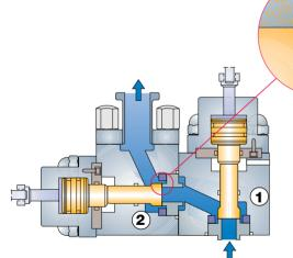
Fig. 6.3.6 Two-stage homogenisation head.
