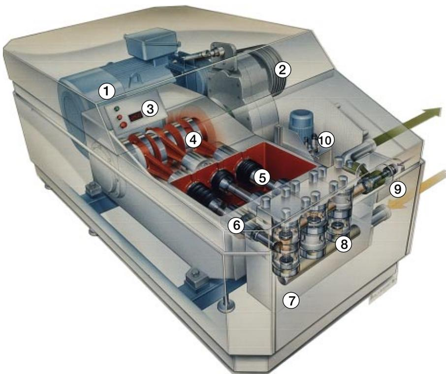
**Fig. 6.3.4** The homogeniser is a large high-pressure pump with a homogenising device.
