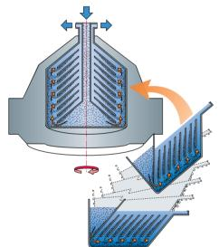
**Fig. 6.2.15** The baffled vessel can be turned 90° and rotated, creating a centrifuge bowl for continuous separation of solid particles from a liquid.
