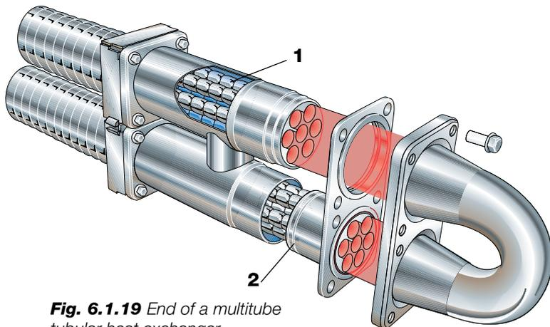
**Fig. 6.1.19** End of a multitube tubular heat exchanger.
