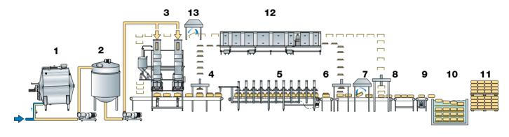
Fig. 14.36 Flowchart for mechanised production for Gouda cheese.
