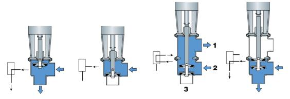
**Fig. 6.8.7** Shut-off and change-over valves with the plug in different positions and the corresponding flow chart symbols.
