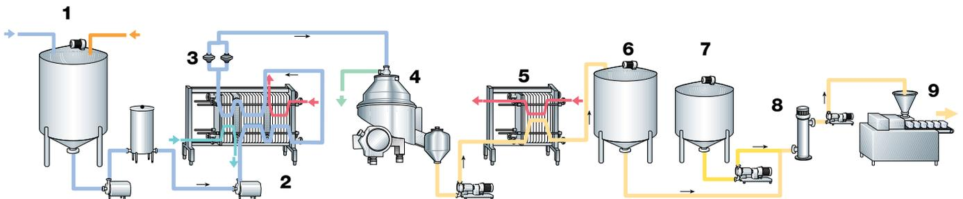
**Fig. 14.44** Flowchart for mechanised production of Quarg
