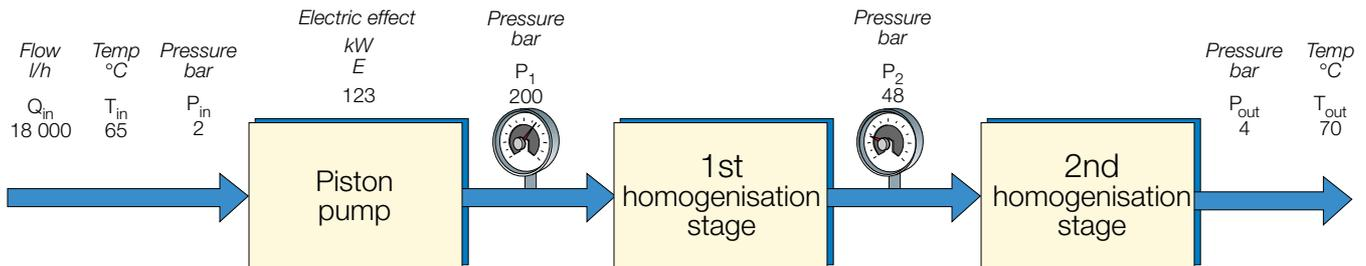
**Fig. 6.3.9** Energy, temperature and pressure in a homogenisation example.
