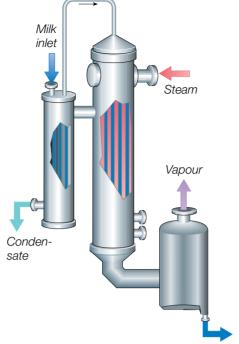
Fig. 6.5.4 Single-effect falling film evaporator.
