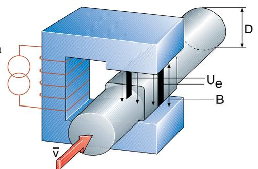
Fig. 6.2.38 Flow transmitter.
