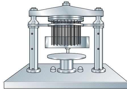
**Fig. 14.40** Pinching machine for piercing blue cheese.
