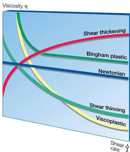
**Fig. 3.5** Viscosity curves for Newtonian and non-Newtonian fluids.
