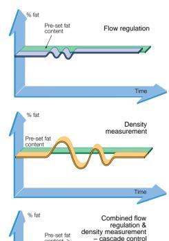
**Fig. 6.2.36** Differences in reaction time between different control systems.
