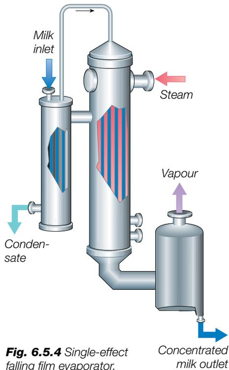
**Fig. 6.5.4** Single-effect falling film evaporator.
