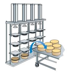
Fig. 14.22 Vertical pressing unit with pneumatically operated pressing plates.
