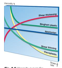
Fig. 3.5 Viscosity curves for Newtonian and non-Newtonian fluids.
