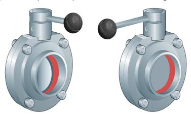
Fig. 6.8.10 Manually controlled butterfly valve in open position (left) and in closed position (right).
