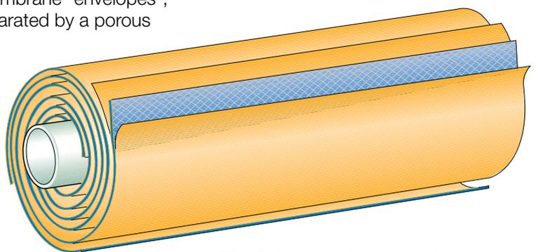
**Fig. 6.4.11** Envelope formation of the spiral-wound filter design.
