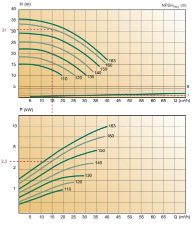
Fig. 6.7.3 Pump chart for a centrifugal pump.
