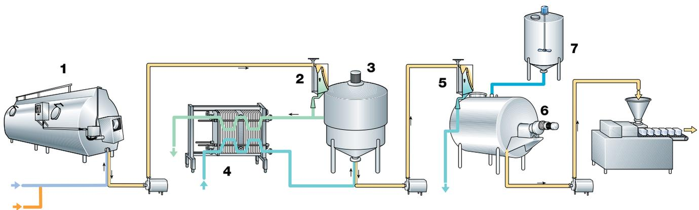
**Fig. 14.43** Flowchart for mechanised production of Cottage cheese.
