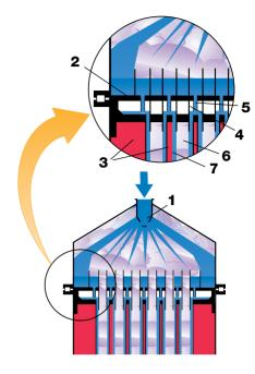
**Fig. 6.5.5** Upper section of a falling film evaporator.
