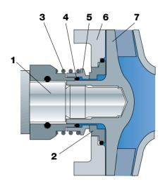
Fig. 6.7.4 Single mechanical shaft seal
