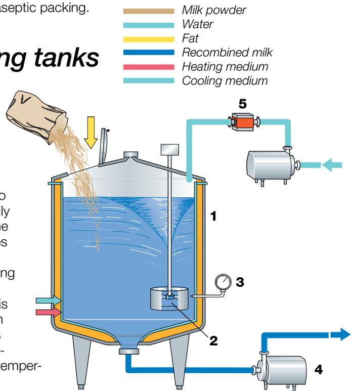
**Fig. 18.4** Recombination plant for batch processing.
