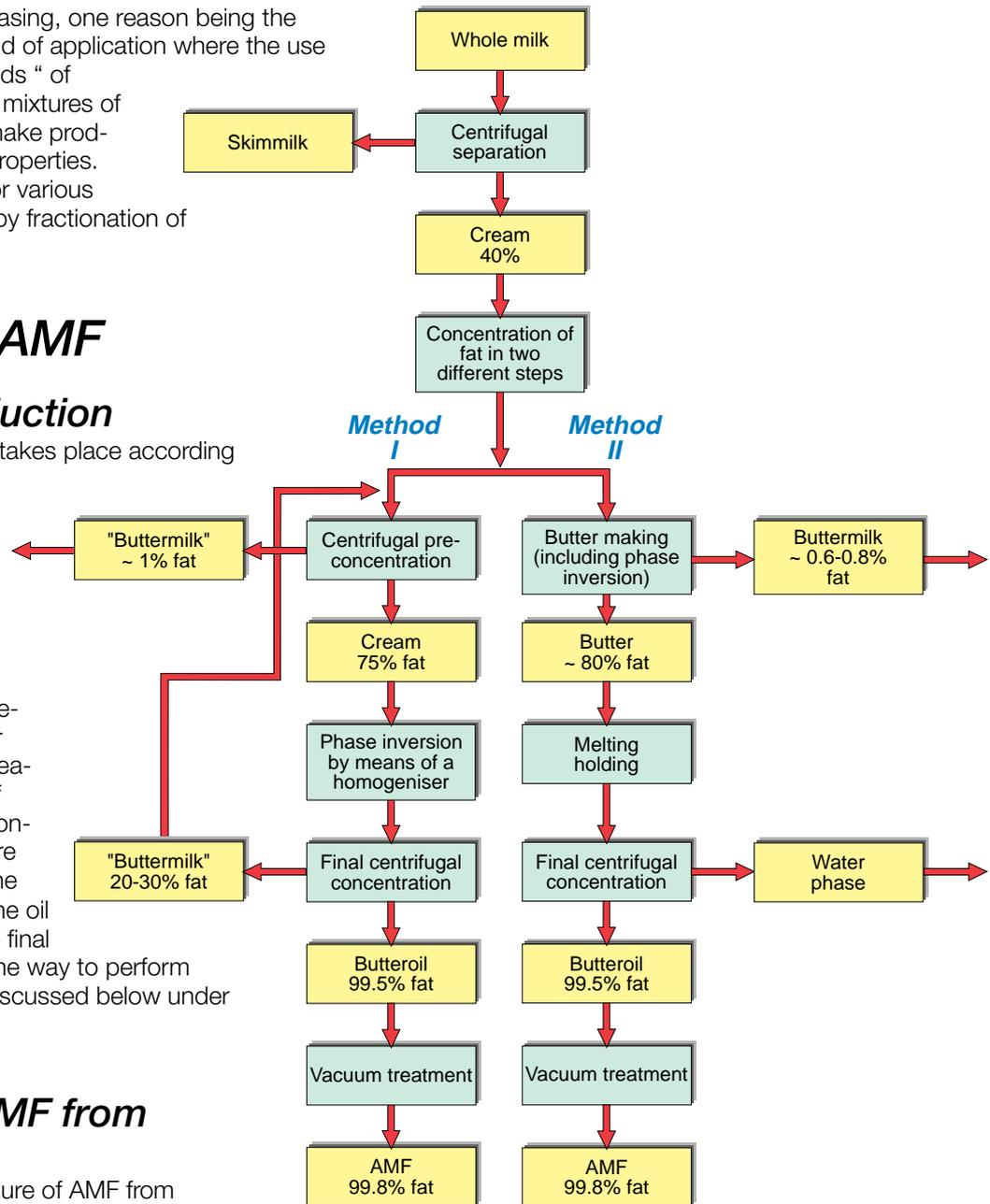
Fig. 13.2 Block chart showing principle of AMF production.
