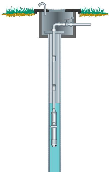
**Fig. 6.11.2** Pipe well with submersible pump.
