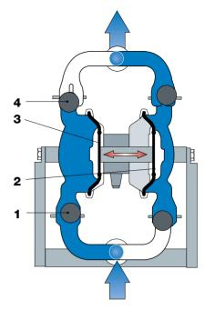
Fig. 6.7.16 The diaphragm pump.
