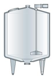
**Fig. 6.9.3** A typical storage tank has a capacity of 1 000 litres up to about 50 000 litres.
