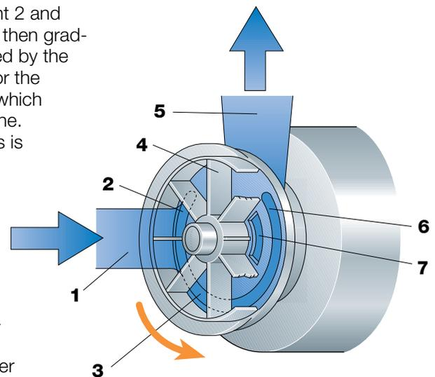
Fig. 6.7.11 Working principle of a self-priming liquid-ring pump.
