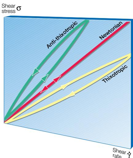
**Fig. 3.6** Flow curves for time-dependant non-Newtonian fluids.
