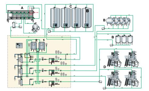
**Fig. 21.5** Principle of the centralised CIP system.
