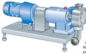
**Fig. 6.7.12** Positive displacement pump of the lobe-rotor type with geared motor assembled on a frame.
