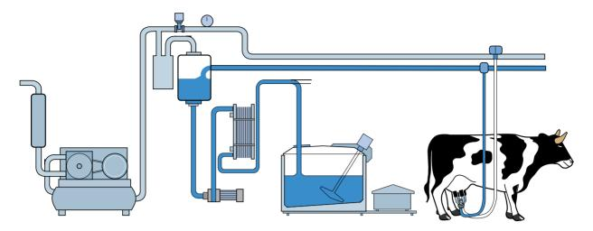
**Fig. 1.12** Milking equipment on a large farm with heat exchanger for rapid chilling from 37 to  $4^{\circ}$ C.
