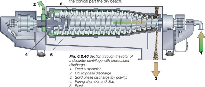
The shell sections are usually ribbed or grooved on the inside to prevent the solids from sideslipping as the conveyor rotates.
