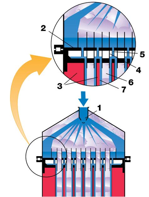
**Fig. 6.5.5** Upper section of a falling film evaporator.
