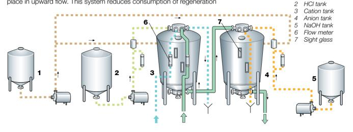
chemicals by as much as 30—40%, but at the expense of a more complicated design. The plant can easily be automated. Two or three parallel ion exchange systems are needed for a continuous flow of whey. A normal cycle time is six hours, four of which are used for regeneration.
