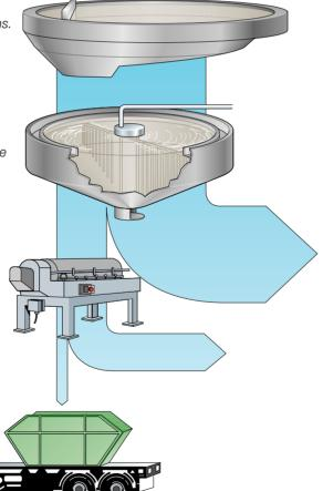
**Fig. 22.5** Reduction in volume of wet sludge from the primary settling stage after treatment in a sludge thickener and decanter centrifuge. The amount of dewatered sludge discharged from the decanter centrifuge is only 8% of the volume of the wet sludge from the sedimentation basins.
