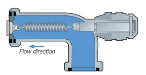
Fig. 6.8.17 Pressure relief valve.
