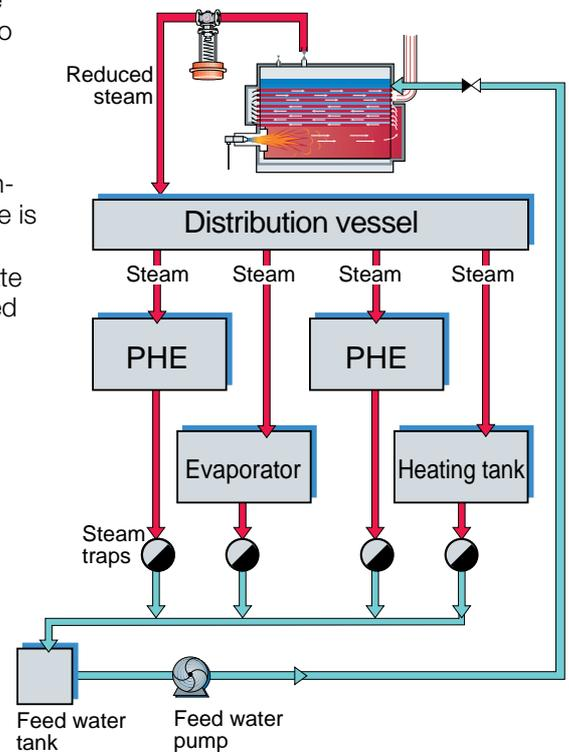
**Fig. 6.11.7** System for steam distribution and condensate collection.
