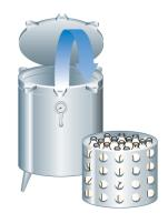
The rotary methods have an advantage over the static method due to the quicker uptake of heat from the heating medium and the greater uniformity of treatment with respect to bacterial kill and colour of finished product.
