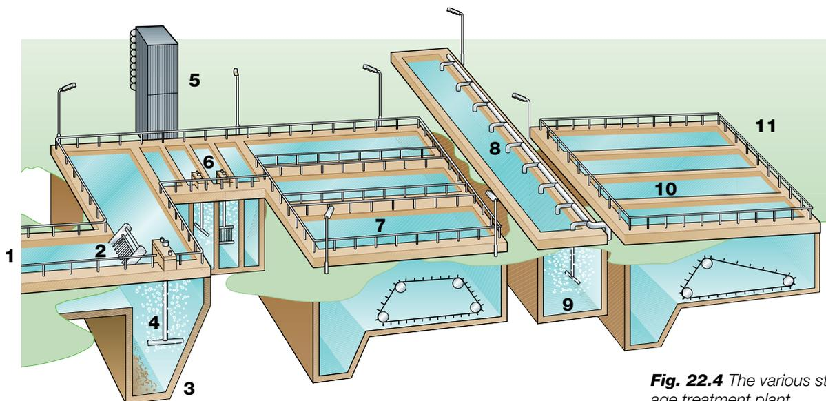
**Fig. 22.4** The various stages of a sewage treatment plant.
