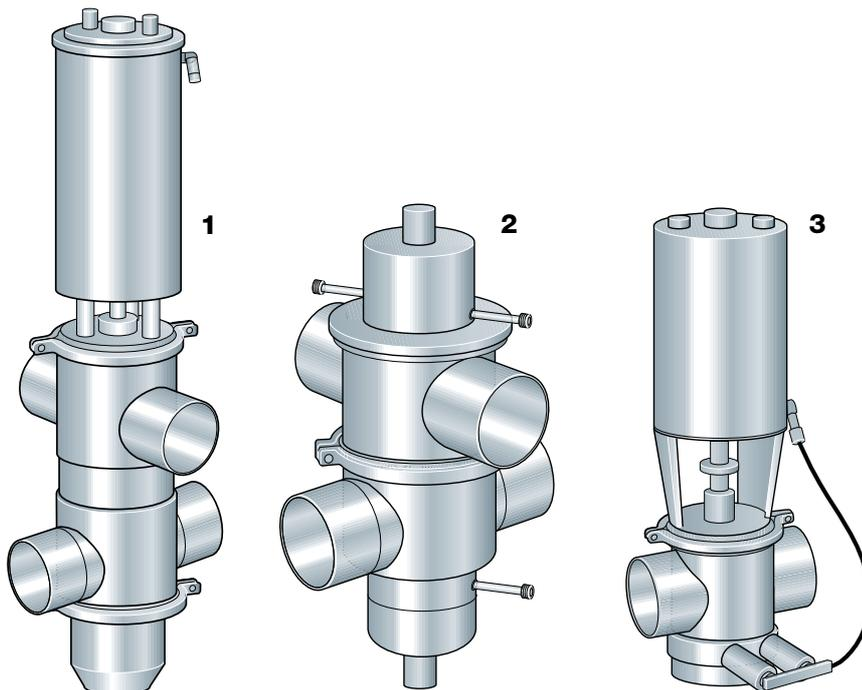
**Fig. 6.8.14** Three types of mixproof valves.
