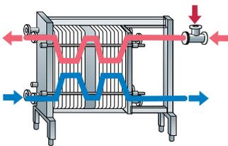
**Fig. 9.14** Plate heat exchanger for heating and cooling.
