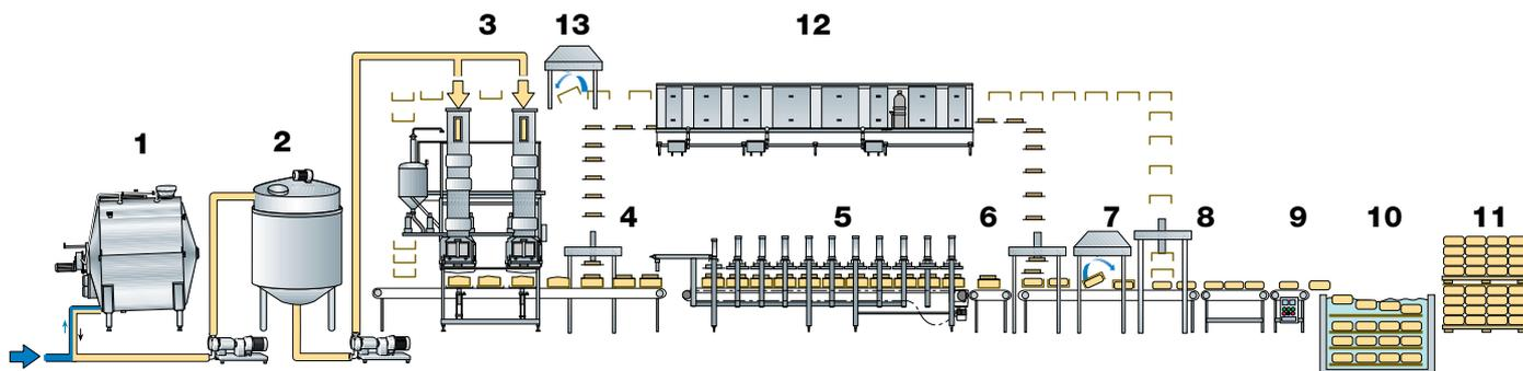
**Fig. 14.36** Flowchart for mechanised production for Gouda cheese.
