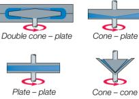
**Fig. 3.9** Operating principles of different types of viscometer.
