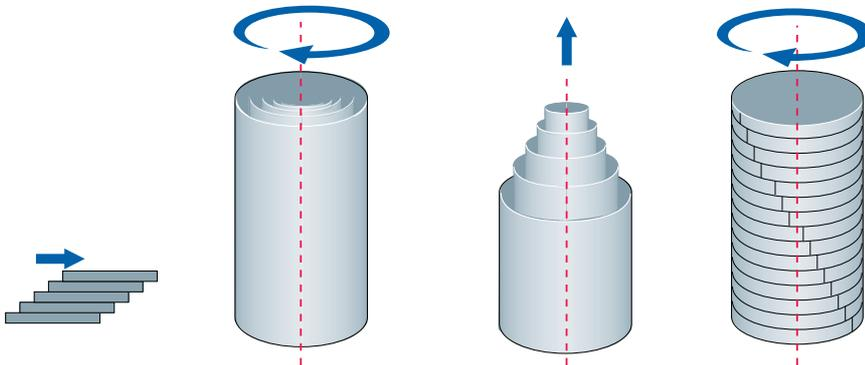
**Fig. 3.2** Different types of shearing.
