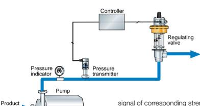
tures, pressures, concentrations and pH values at certain predetermined magnitudes. The equipment for monitoring and controlling these parameters comprises various types of transmitters, controllers and control equipment. In figure 7.12 a control loop is illustrated.
