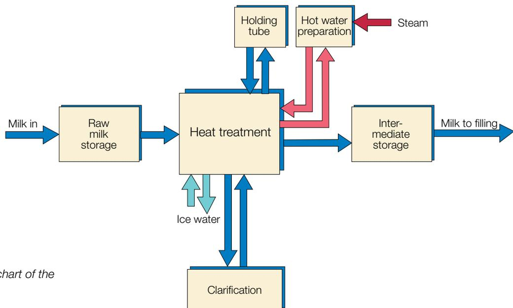
**Fig. 7.1** Generalised block chart of the milk pasteurisation process.
