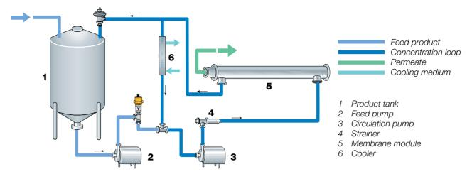
Fig. 6.4.17 Batch membrane filtration plant
