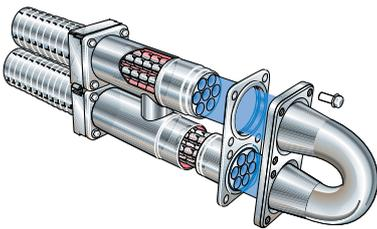
**Fig. 9.15** Tubular heat exchanger for heating and cooling.
