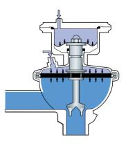
Fig. 6.8.22 Constant-pressure modulating valve with a booster for control of products with a higher pressure than the available air pressure.
