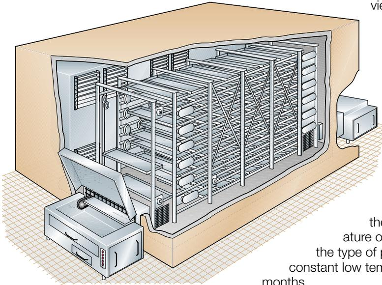
**Fig. 19.8** Hardening tunnel.
