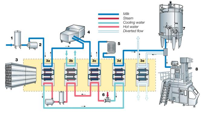
Indirect UHT plant based on scraped surface heat exchangers
