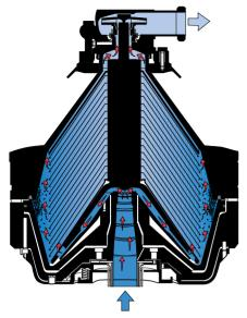
Fig. 7.6 Bowl of a centrifugal clarifier.
