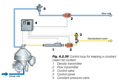
is that the density will vary with the degree of crystallisation and will thus jeopardise the measuring accuracy of the density transmitter, which is always calibrated at prevailing conditions after having been installed.
