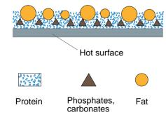
Fig. 21.1 Deposits on a heated surface.
