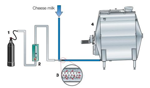
**Fig. 14.8** Addition of CO<sub>2</sub> gas to cheese milk.
