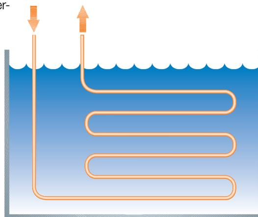
**Fig. 6.11.11** Ice water tank with evaporator coils.
