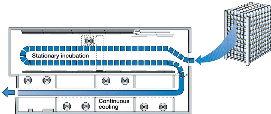
**Fig. 11.19** Combined incubation room and cooling tunnel.
