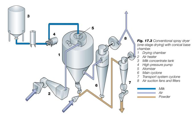
that all removal of moisture from the concentrate to the required final moisture content takes place in the spray drying chamber (1). The subsequent pneumatic conveying system serves only to collect the powder leaving the chamber cone together with the powder fraction separated from the exhaust air in the main cyclone (6), to cool the powder and feed it via the final cyclone (7) to the bagging-off hopper.
