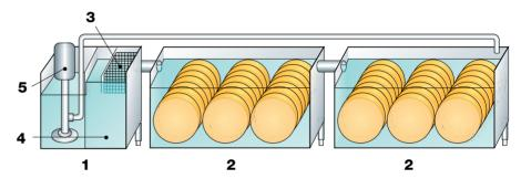
Fig. 14.28 Brine bath system with containers and brine circulation equipment.
