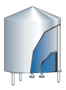
Fig. 11.10 Tubular holding section.
