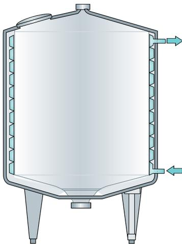
**Fig. 6.9.4** Mixing tank with welded-on heating/cooling channels.
