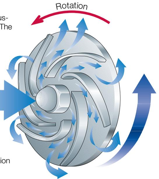
**Fig. 6.7.6** Flow principle in a centrifugal pump.
