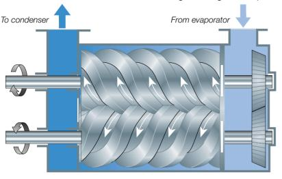
Fig. 6.11.12 Design principle of the screw compressor.
