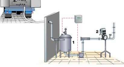
Fig. 6.6.3 Milk reception at the dairy with air eliminator (1) and volume measuring device (2)
