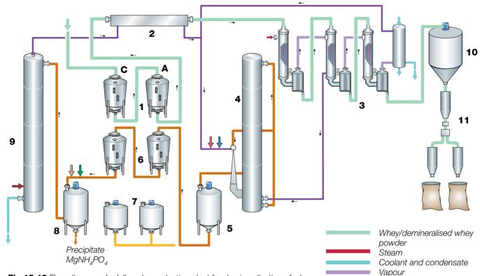
Fig 15.13 Flow diagram of a full-scale production plant for demineralisation of whey powder.
