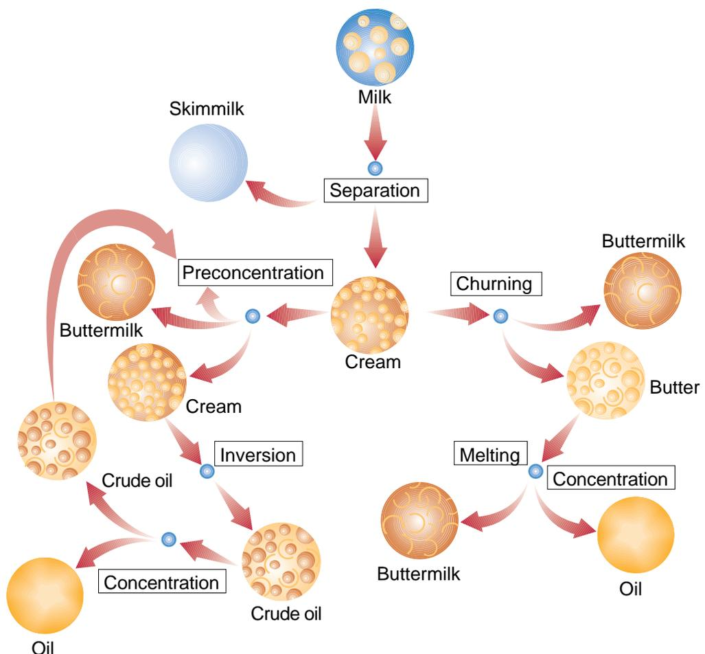
**Fig. 13.1** Basics of AMF production: Concentration of milk fat, phase inversion, concentration of oil.
