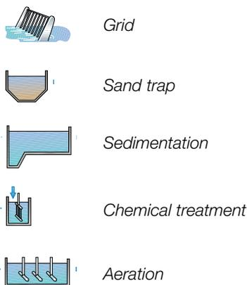
**Fig. 22.3** The various stages of sewage treatment can be combined in several ways.
