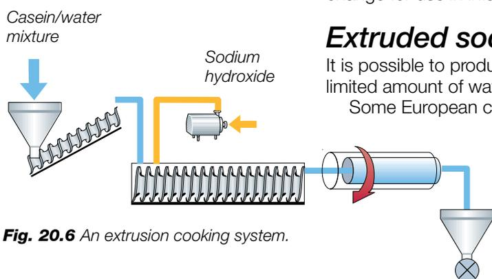
Fig. 20.6 An extrusion cooking system.
