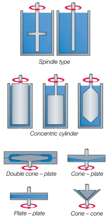
**Fig. 3.9** Operating principles of different types of viscometer.
