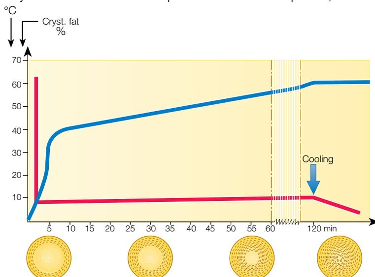
**Fig. 8.4** The crystallisation process for 40% cream at  $8^{\circ}\text{C}$ .
