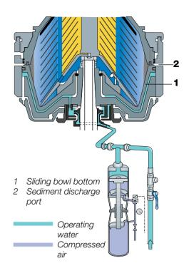
**Fig. 6.2.30** The valve system supplying operating water to a separator in order to guarantee proper discharge performance.
