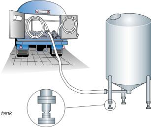
Fig. 5.13 Milk reception via a weighing tank
