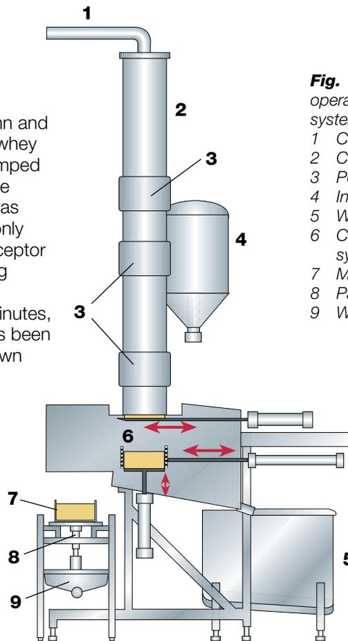
**Fig. 14.17** Casomatic, an intermittently operating continuous pre-pressing system, supplemented with mould filler.
