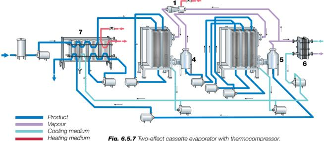
Fig. 6.5.7 Two-effect cassette evaporator with thermocompressor.
