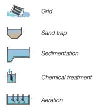
**Fig. 22.3** The various stages of sewage treatment can be combined in several ways.
