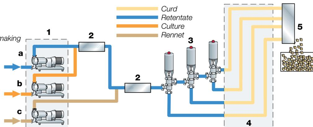
filled. The proper coagulation time in the pipes is controlled by the speed of the dosing pump.
