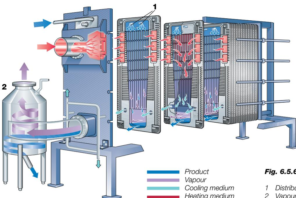
**Fig. 6.5.6** Plate type cassette evaporator.
