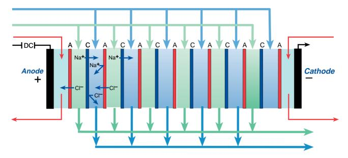
Fig. 15.9 Cell packs for electrodialysis.
