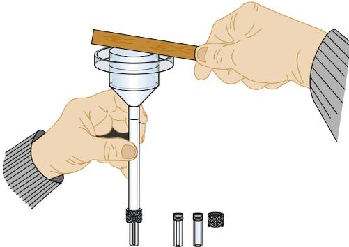
Fig 11.8 The SMR viscosimeter.
