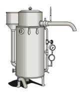
Fig. 6.1.13 This type of flash pasteuriser with a turbine-driven stirrer was manufactured and sold by AB Separator between 1896 and 1931.
