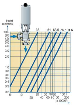
**Fig. 7.11** Pressure-drop graph for a shut-off valve.
